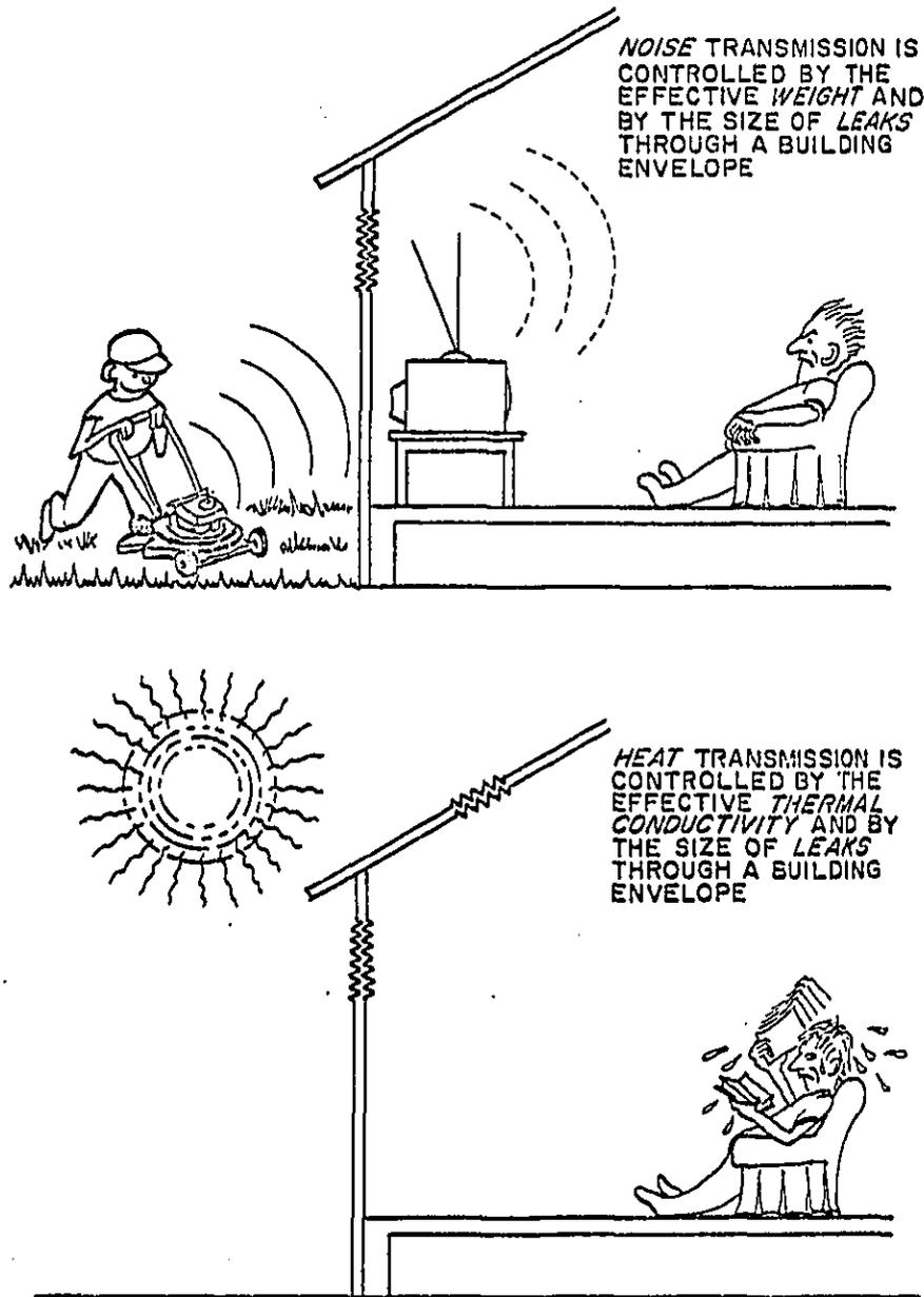
FIG. 1.1 PROPERTIES OF BUILDING ENVELOPES AFFECTING NOISE TRANSMISSION AND ENERGY CONSUMPTION.
