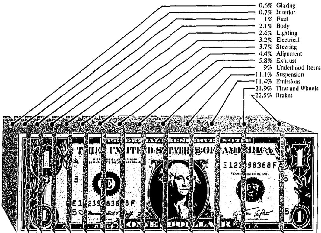
Figure 28: Distribution of Vehicle System Repair Costs
