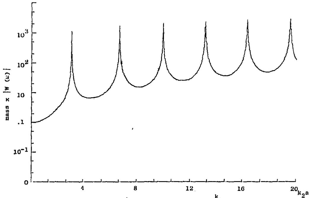
FIGURE 10: mass x  $|W(\omega)|$  rotational wave alone  $\frac{k_1}{k_2} = .01$
