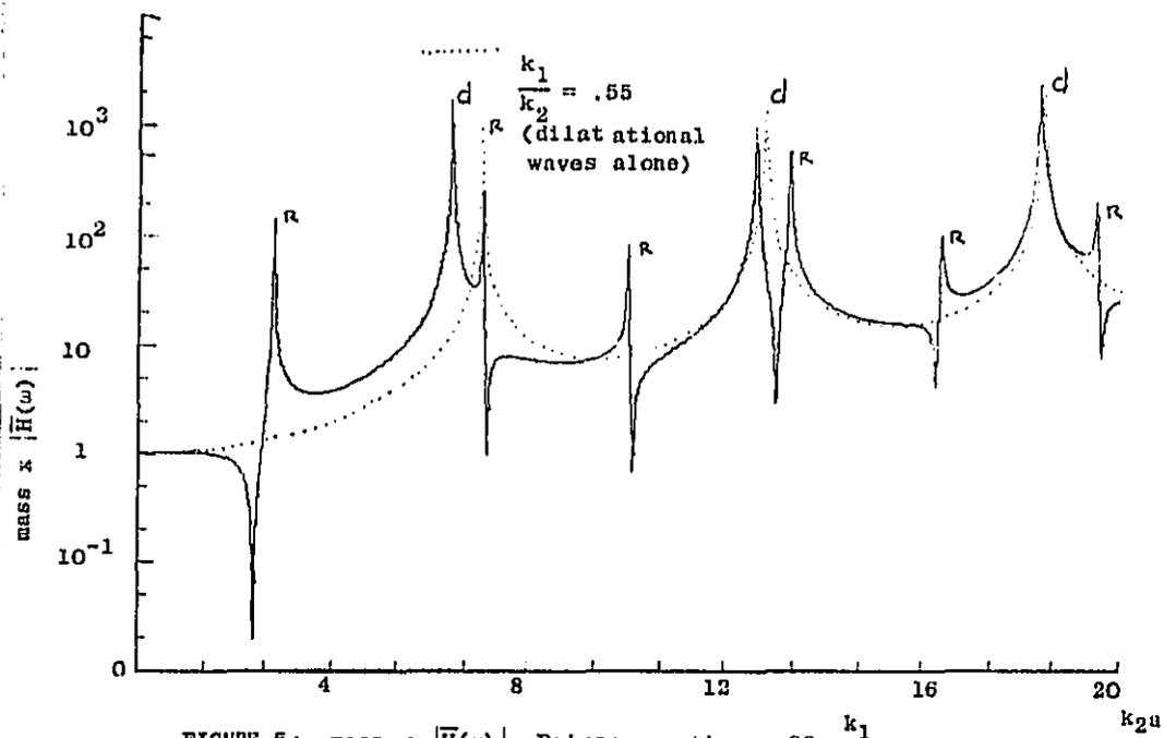
FIGURE 5:  $\text{mass} \times |\bar{H}(\omega)|$ , Poissons ratio = .28,  $\frac{k_1}{k_2} = .55$
