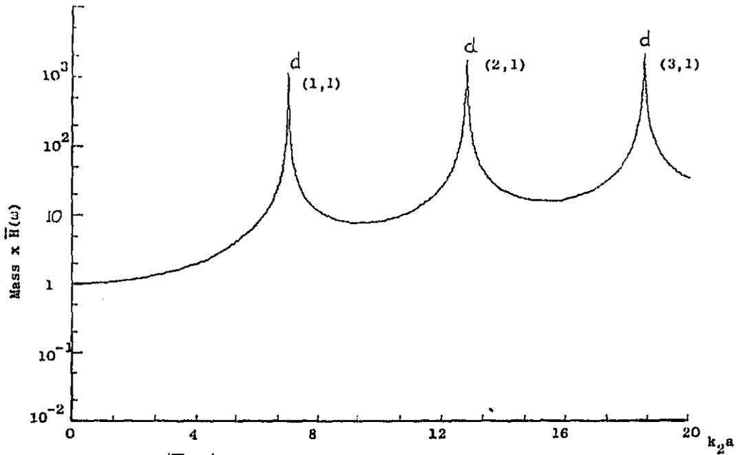
FIGURE 3:  $|\bar{H}(\omega)|$  normalised to the disc mass  $k_1/k_2 = .55$
