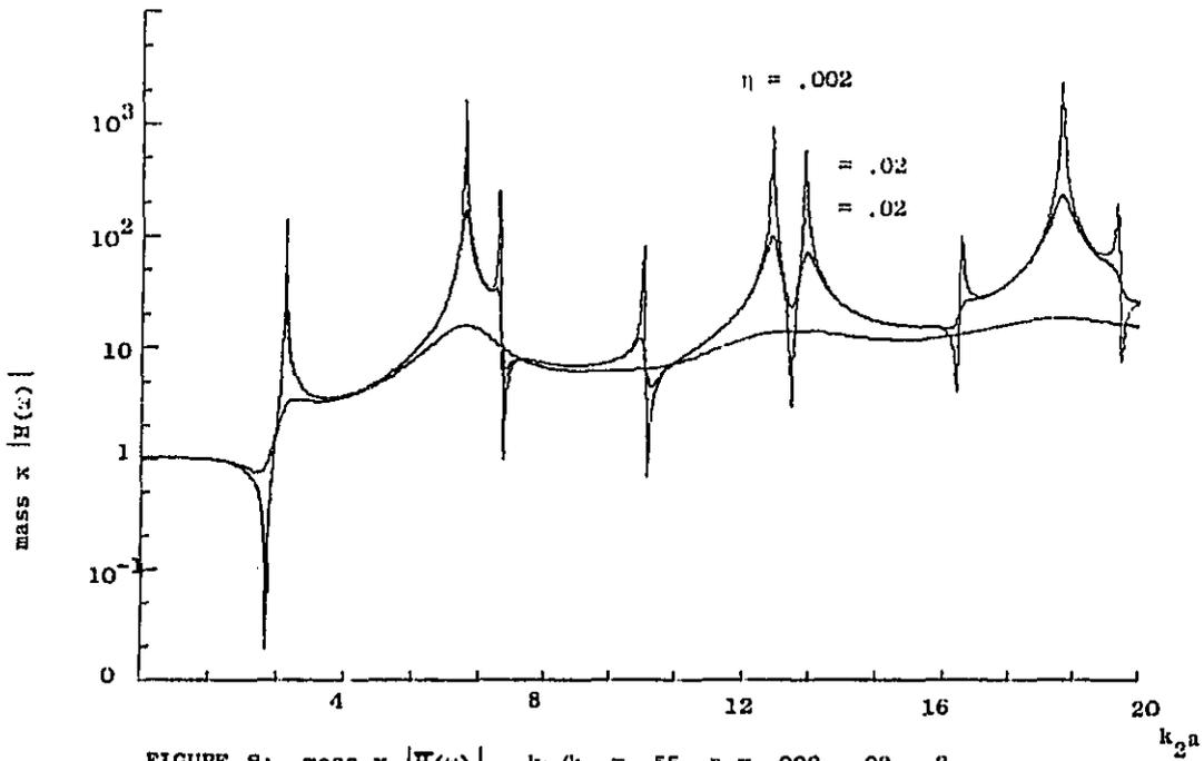
FIGURE 8:  $\text{mass} \times |H(\omega)|$ ,  $k_1/k_2 = .55$ ,  $\eta = .002, .02, .2$
