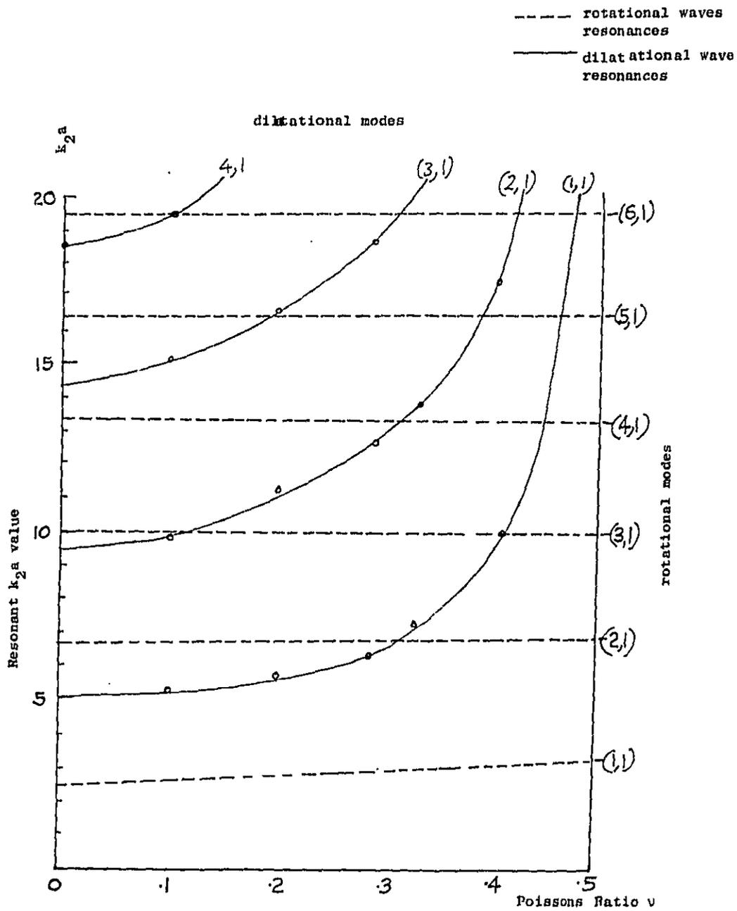
FIGURE 7:  $k_2 a$  resonance values as a function of Poisson's ratio, for a thick disc
