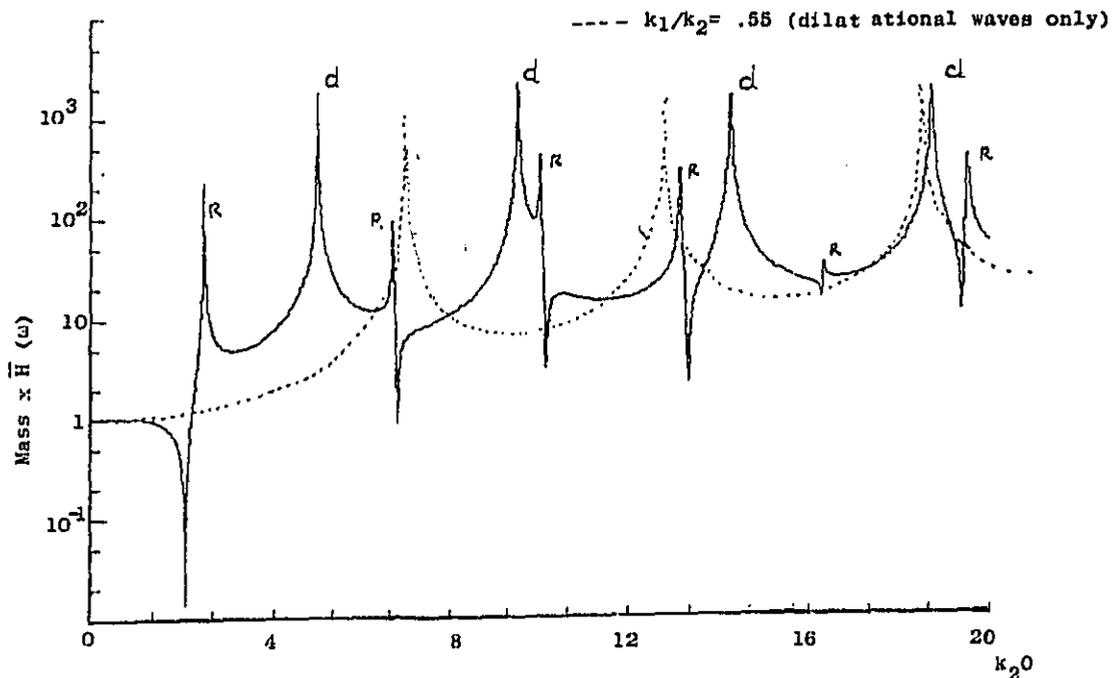
FIGURE 4:  $H(\omega) \times$  disc mass, Poissons Ratio = 0,  $\frac{k_1}{k_2} = .706$
