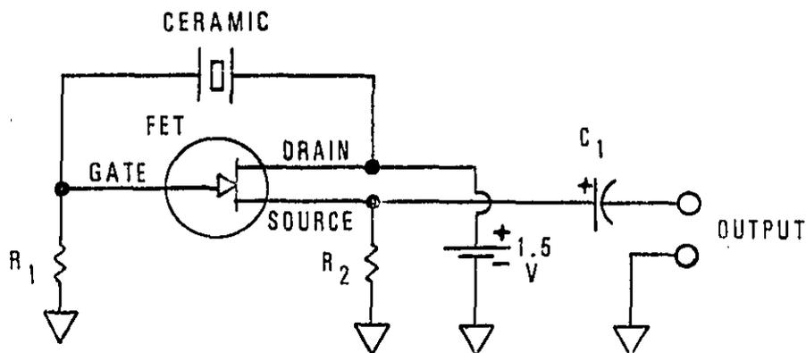
The basic purpose of this circuit is impedance matching. It transforms from the very high impedance of the ceramic sensing element to
