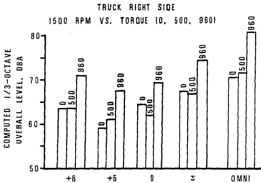
2. Dynamometer Contribution - At some load and engine speeds the dynamometer contributes noise to the omnidirectional microphone but not to the array output level and therefore  $\Sigma$  should not be the same level at the measured omnidirectional level.
