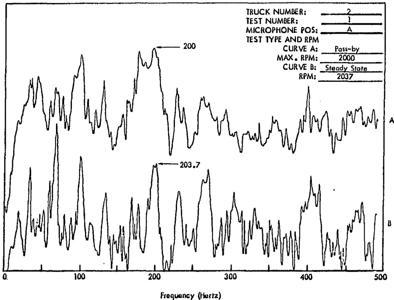
Figure C3 . Truck Exterior Noise Spectra (Narrow Band Analysis 1-1/4 Hertz) Measured at 50 Feet.
