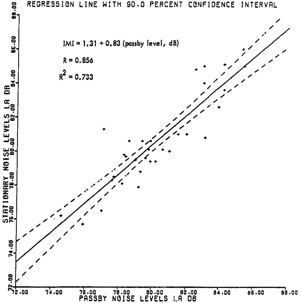
Figure 17. Passby Versus Stationary Test
