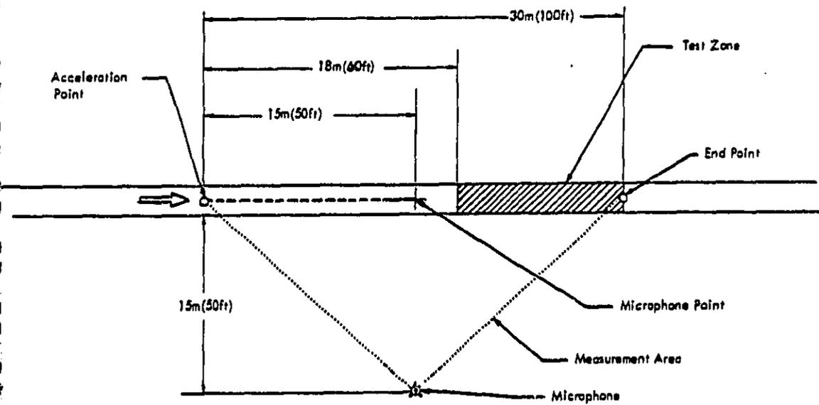
Figure 5. Passby Test Site Configuration and Microphone Position
