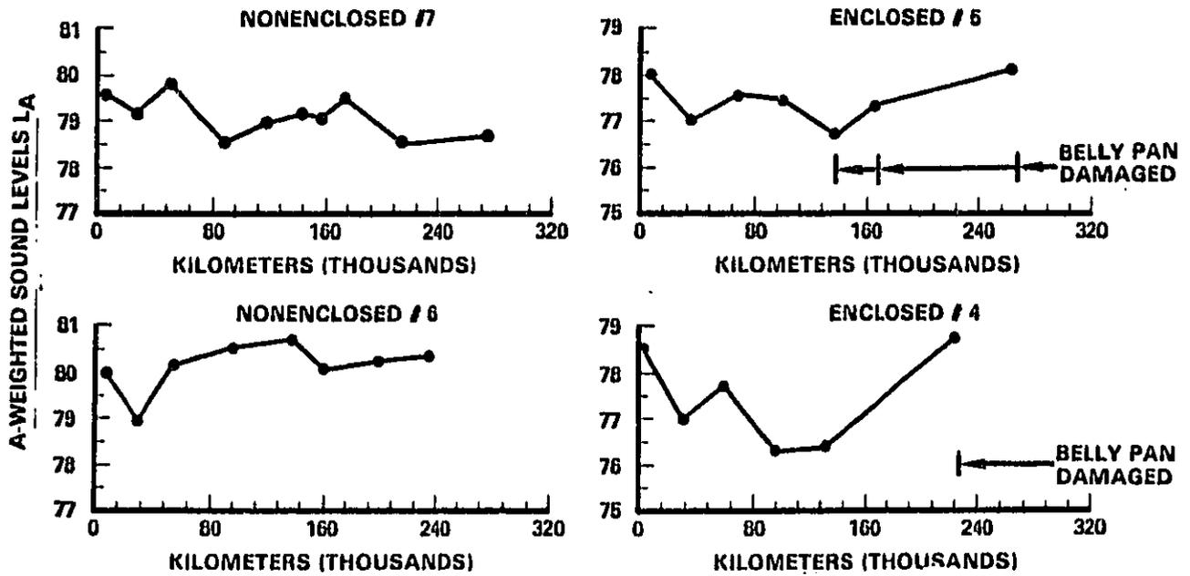
Figure 18. Vehicle Exterior Noise Levels versus Cumulative Kilometers
