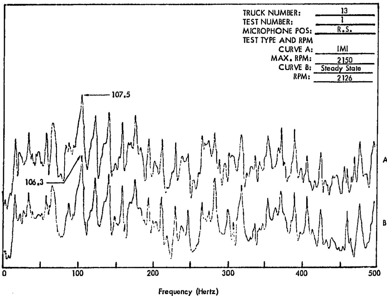
Figure C45 . Truck Exterior Noise Spectra (Narrow Band Analysis 1-1/4 Hertz) Measured at 50 Feet.
