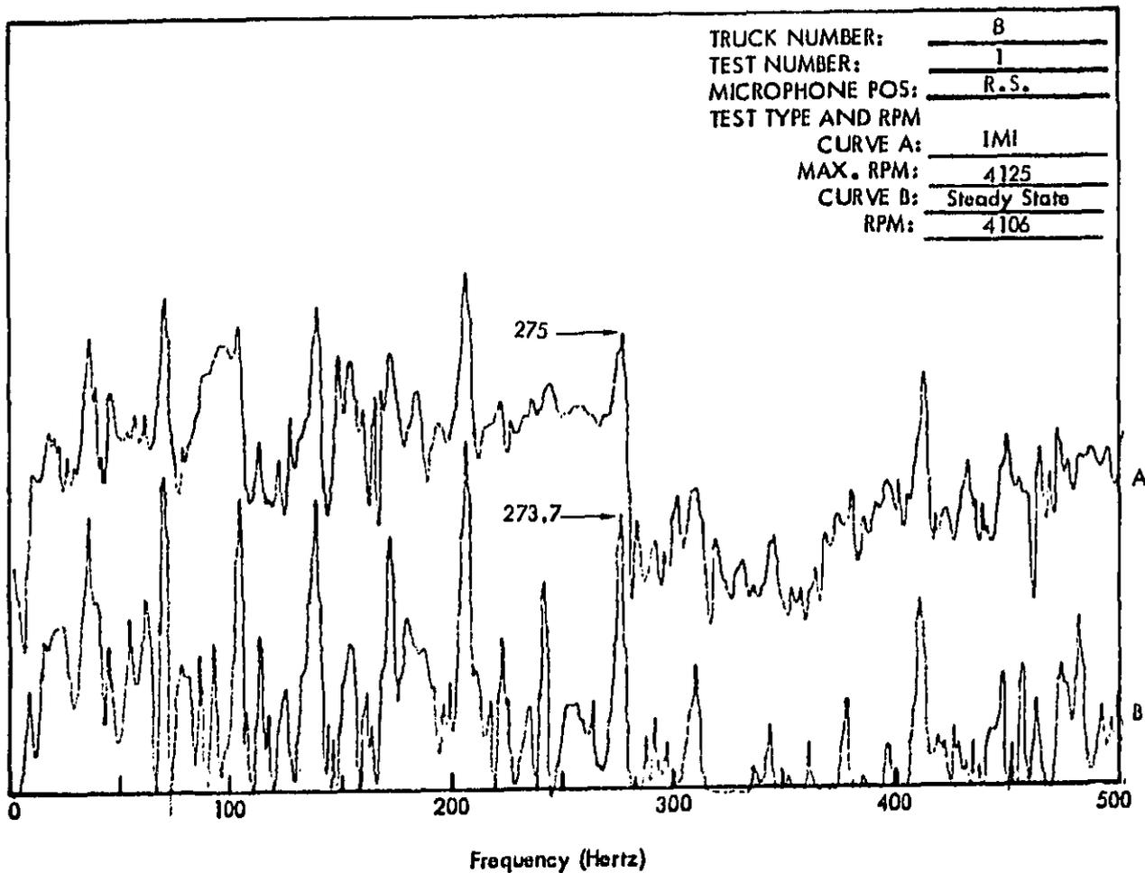
Figure C25. Truck Exterior Noise Spectra (Narrow Band Analysis 1-1/4 Hertz) Measured at 50 Feet. The Spectra Are Used For Determining Engine RPM.
