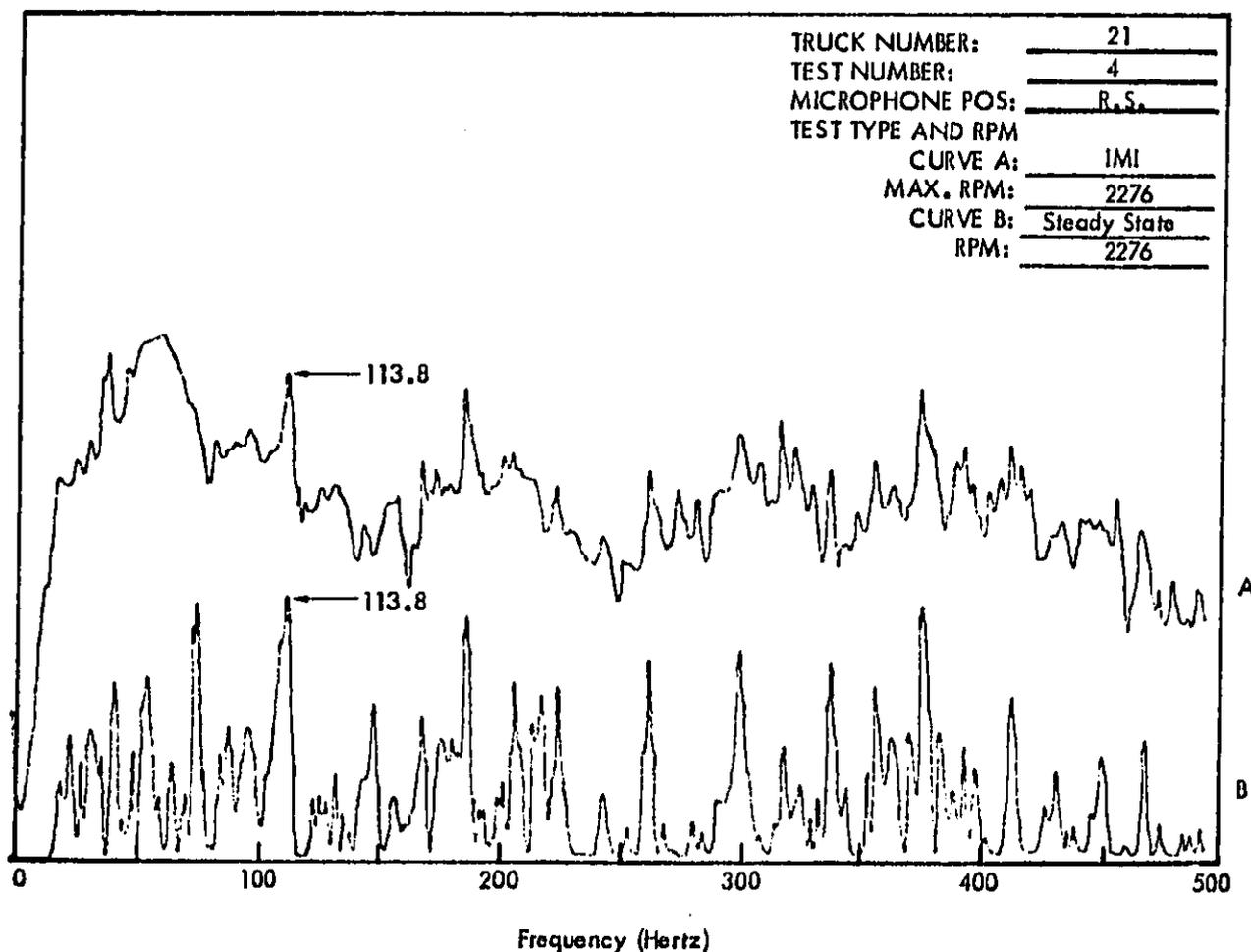
Figure C54. Truck Exterior Noise Spectra (Narrow Band Analysis 1-1/4 Hertz) Measured at 50 Feet.
