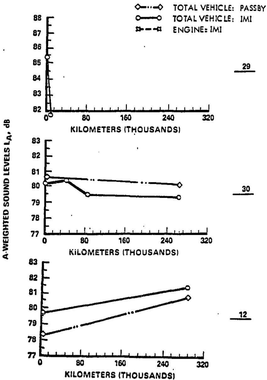
Figure 14. Vehicle Exterior Noise Levels versus Cumulative Kilometers
