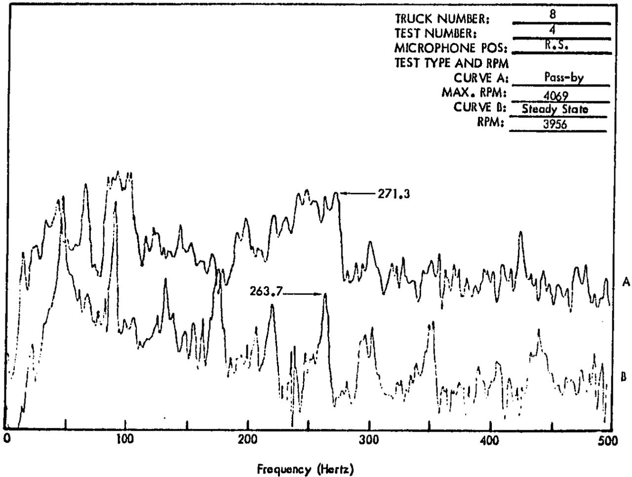
Figure C29. Truck Exterior Noise Spectra (Narrow Band Analysis 1-1/4 Hertz) Measured at 50 Feet.
