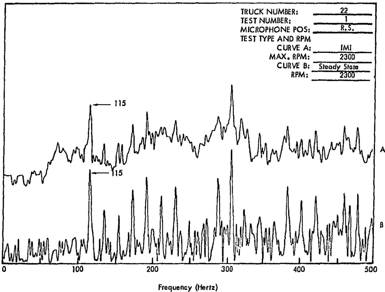
Figure C57 . Truck Exterior Noise Spectra (Narrow Band Analysis 1-1/4 Hertz) Measured at 50 Feet.
