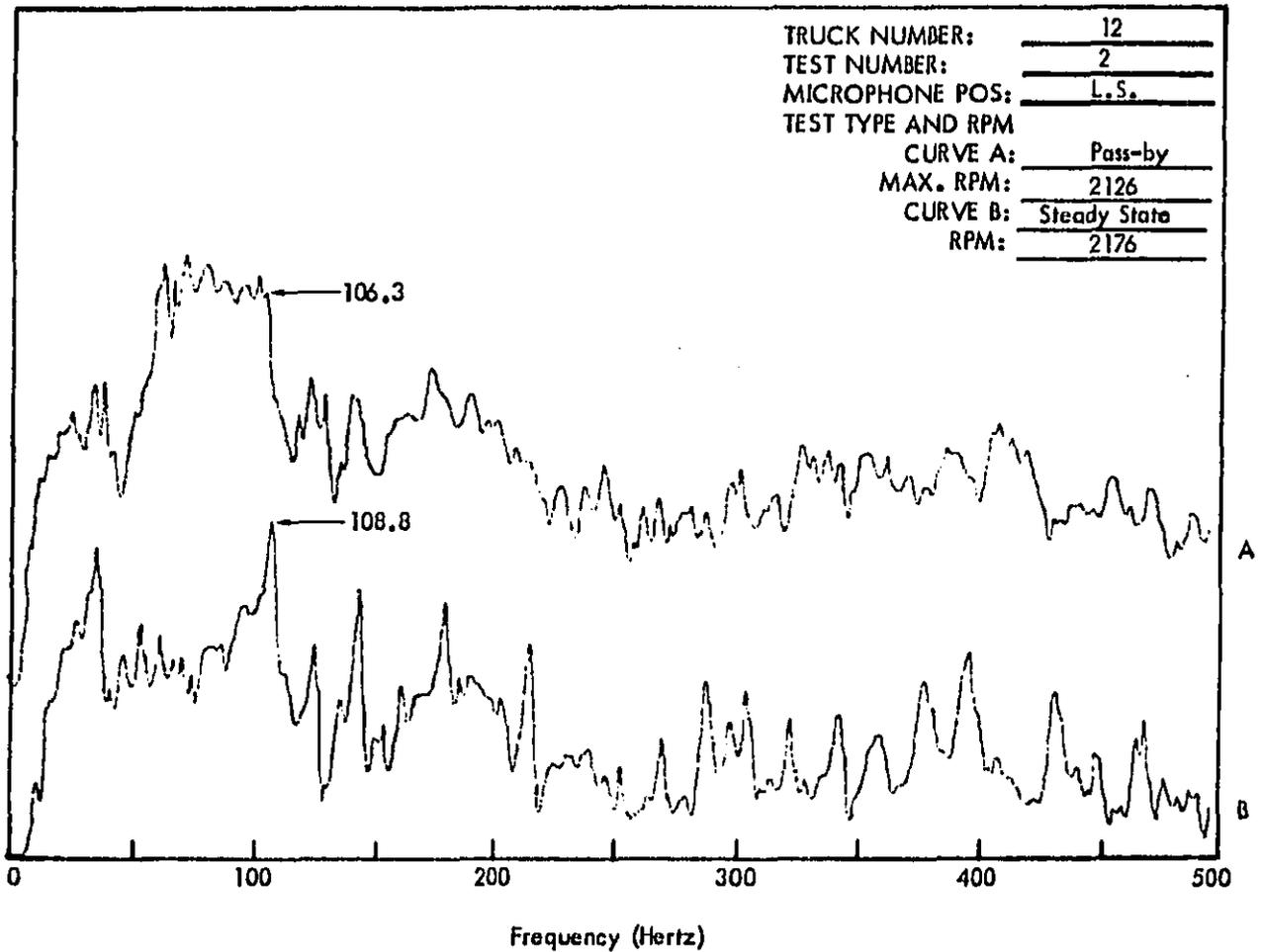
Figure C40. Truck Exterior Noise Spectra (Narrow Band Analysis 1-1/4 Hertz) Measured at 50 Feet.
