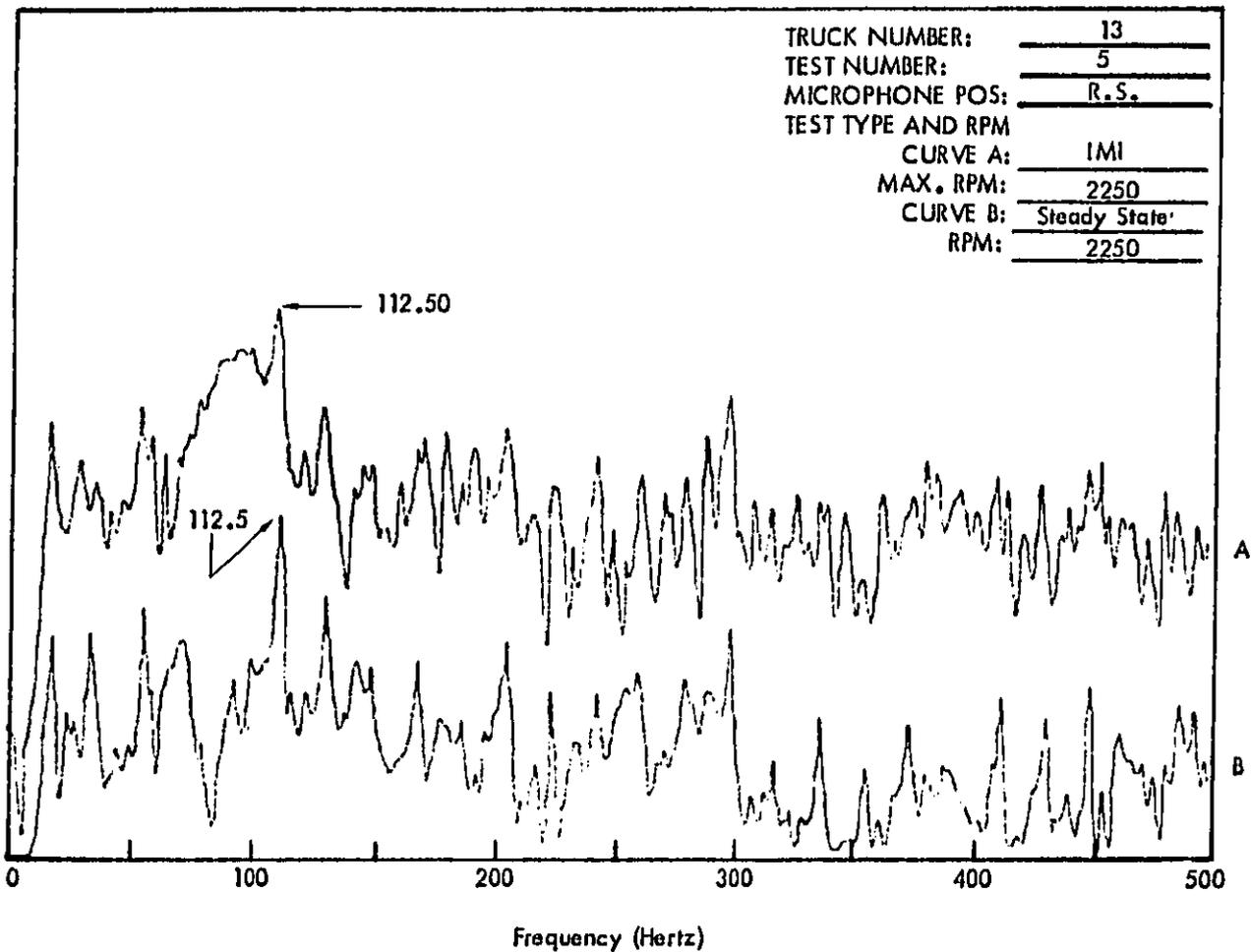
Figure C48. Truck Exterior Noise Spectra (Narrow Band Analysis 1-1/4 Hertz) Measured at 50 Feet.
