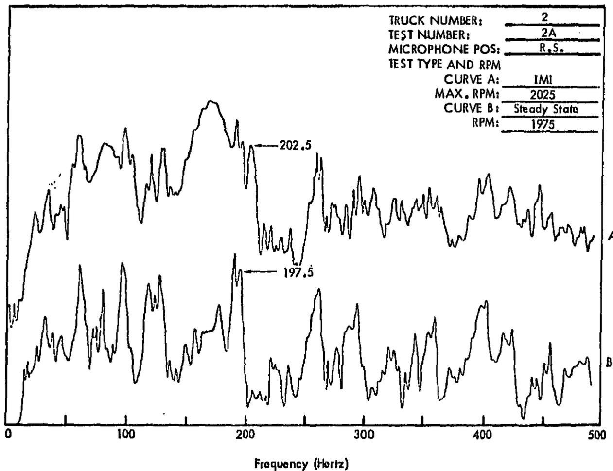
Figure C4 . Truck Exterior Noise Spectra (Narrow Band Analysis 1-1/4 Hertz) Measured at 50 Feet.
