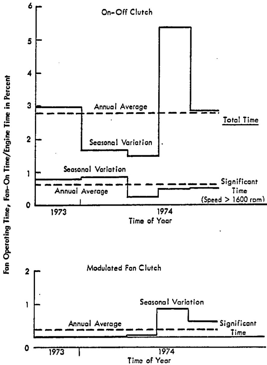
Figure 19. Fan Clutch Operating Time (Reference 5)
