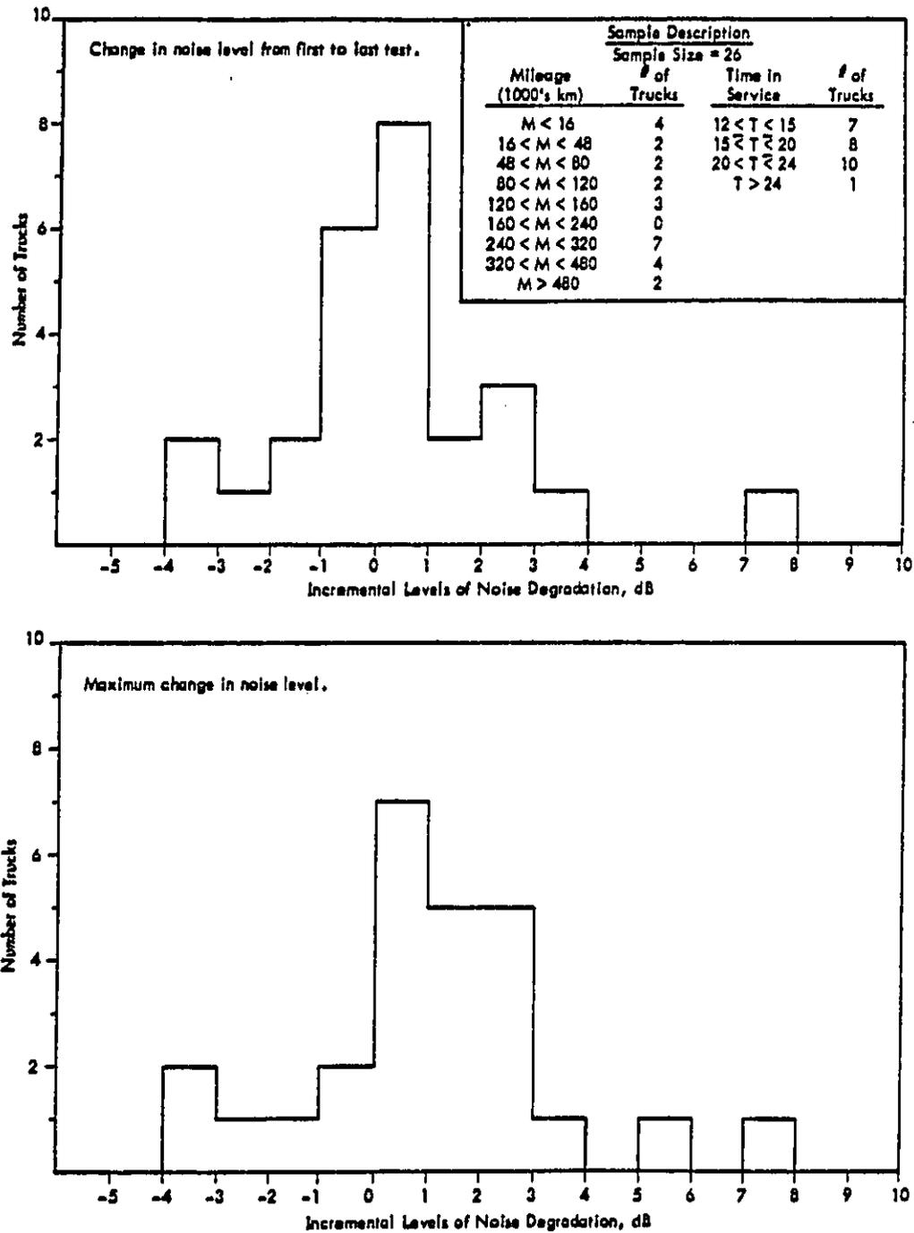
Figure 16. Distribution of Levels of Truck Noise Degradation as Measured Using IMI Stationary Test Procedure
