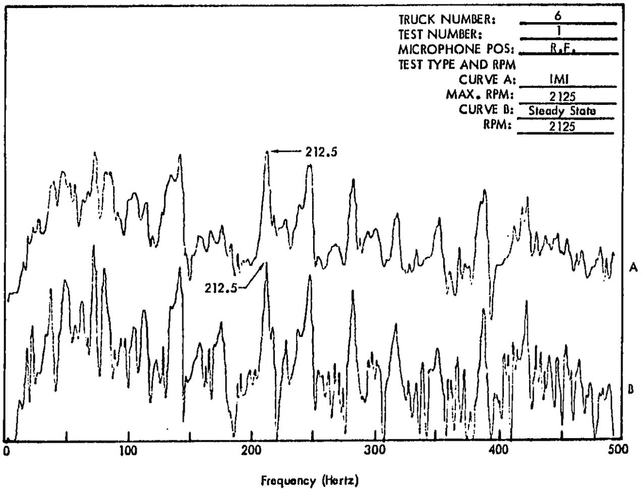
Figure C13. Truck Exterior Noise Spectra (Narrow Band Analysis 1-1/4 Hertz) Measured at 50 Feet.
