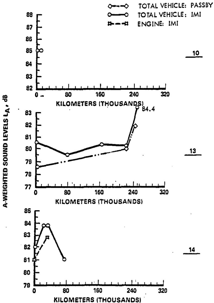
Figure 9. Vehicle Exterior Noise Levels versus Cumulative Kilometers
