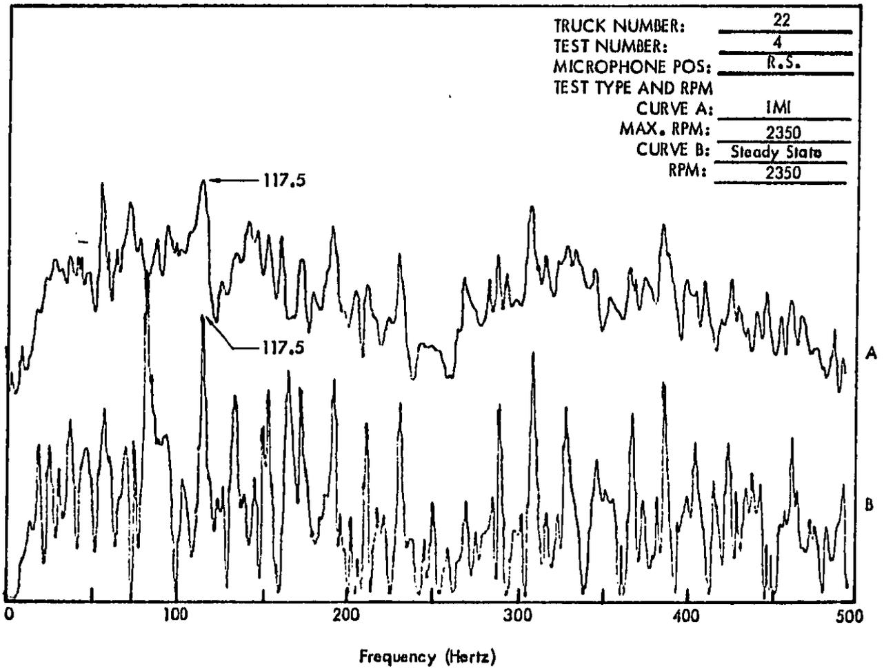
Figure C58 . Truck Exterior Noise Spectra (Narrow Band Analysis 1-1/4 Hertz) Measured at 50 Feet.
