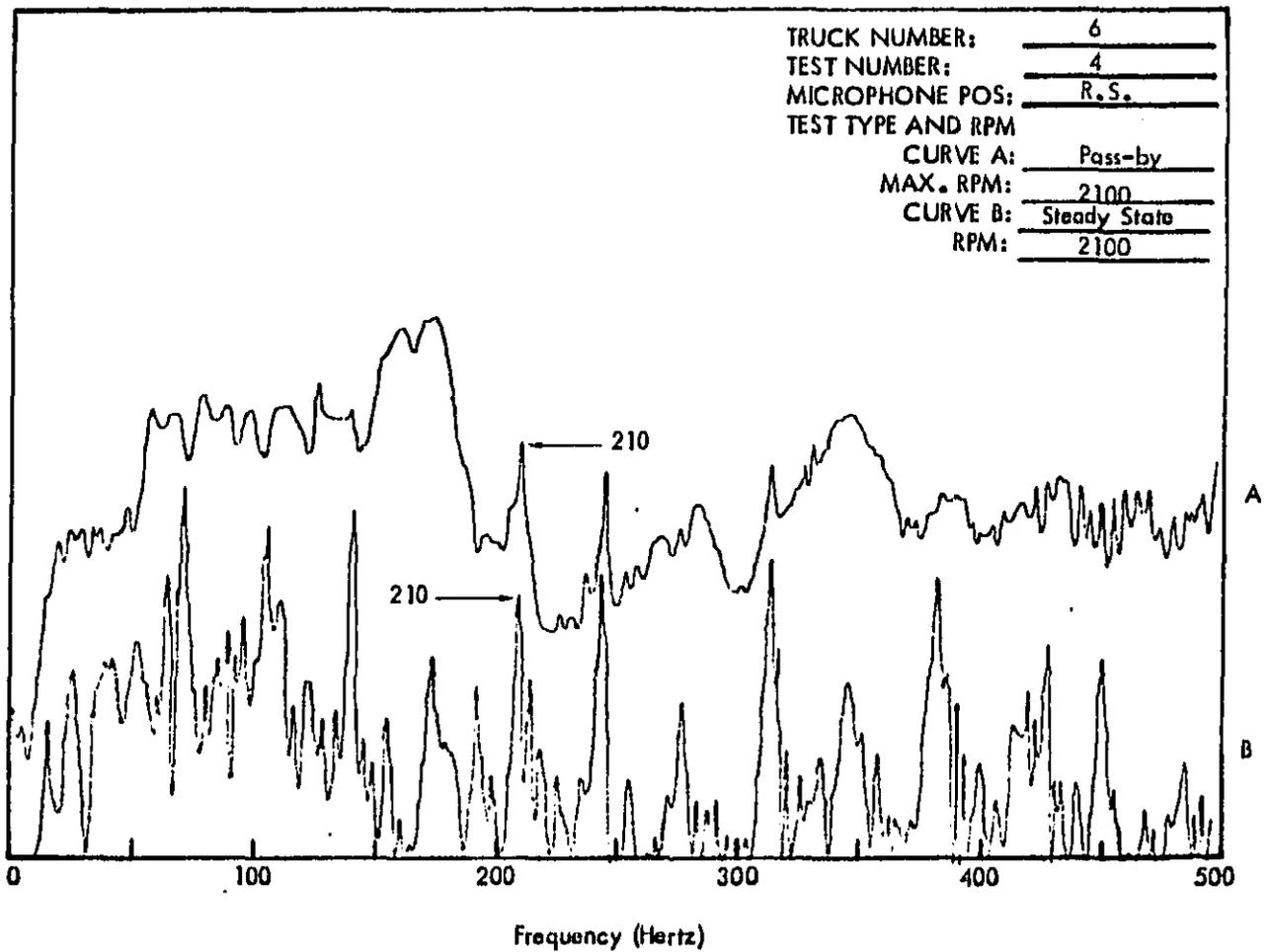
Figure C17. Truck Exterior Noise Spectra (Narrow Band Analysis 1-1/4 Hertz) Measured at 50 Feet.
