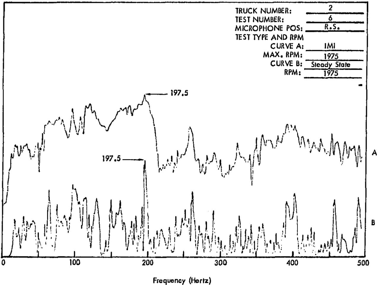
Figure C7 . Truck Exterior Noise Spectra (Narrow Band Analysis 1-1/4 Hertz) Measured at 50 Feet.
