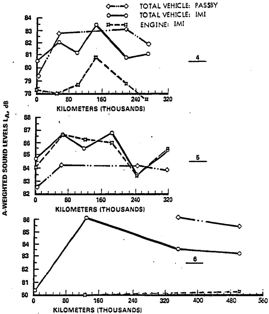
Figure 7. Vehicle Exterior Noise Levels versus Cumulative Kilometers
