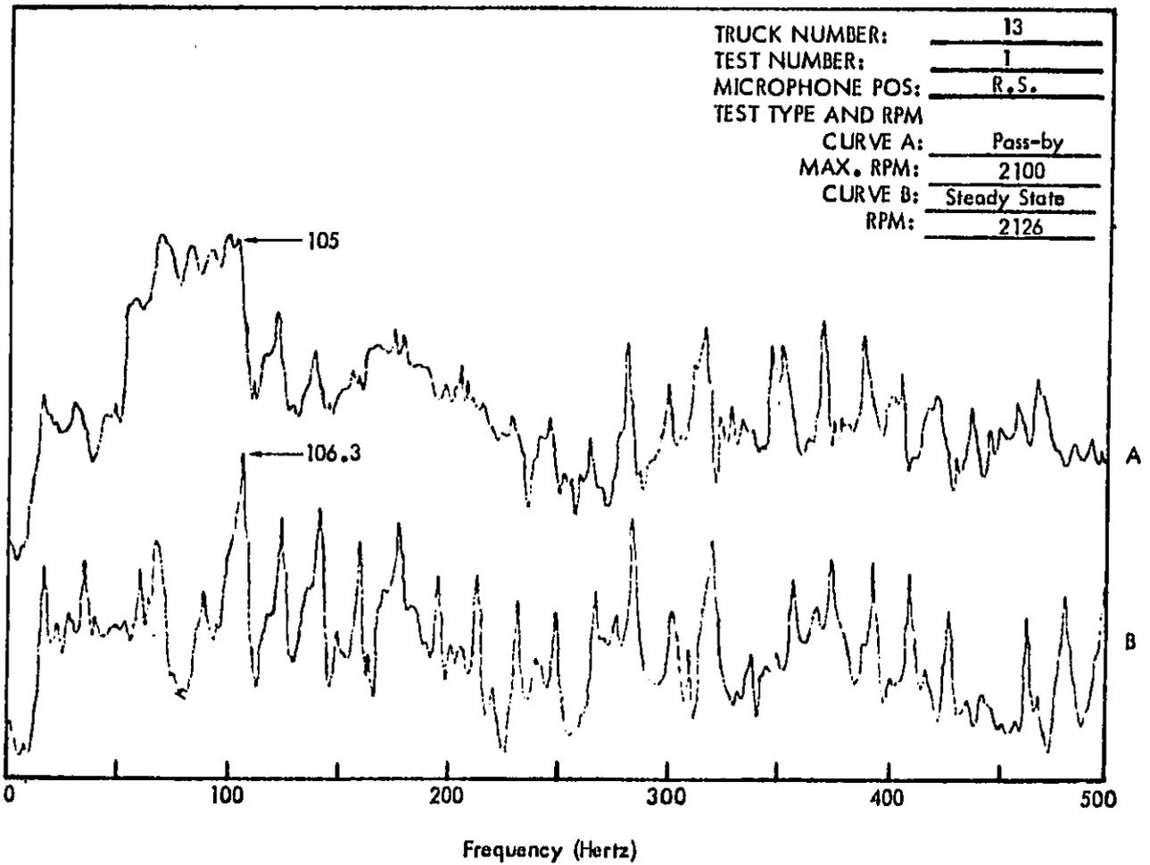
Figure C46 . Truck Exterior Noise Spectra (Narrow Band Analysis 1-1/4 Hertz) Measured at 50 Feet.
