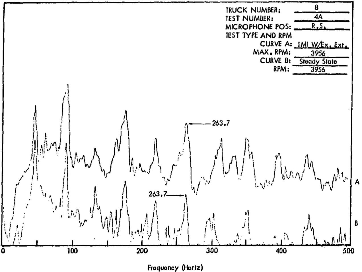
Figure C30. Truck Exterior Noise Spectra (Narrow Band Analysis 1-1/4 Hertz) Measured at 50 Feet.
