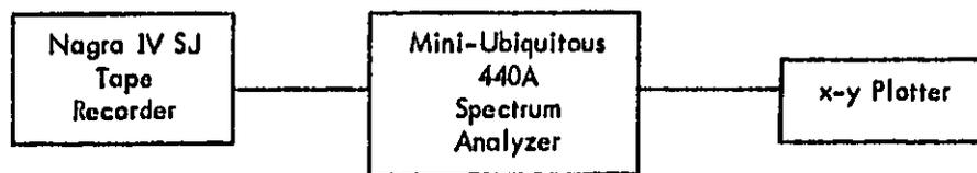
Figure C1. Instrumentation Used for RPM Determination
