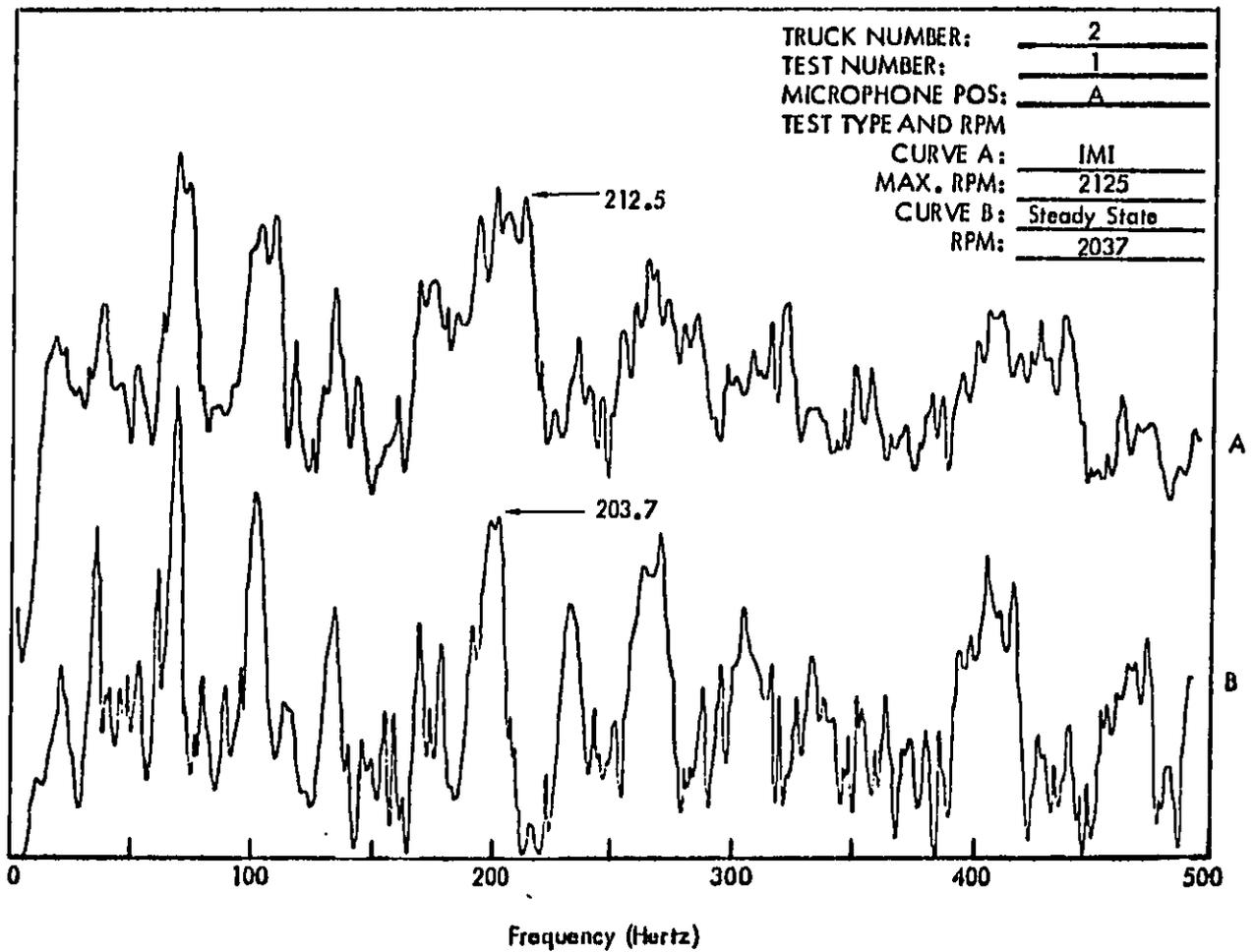
Figure C2 . Truck Exterior Noise Spectra (Narrow Band Analysis 1-1/4 Hertz) Measured at 50 Feet.
