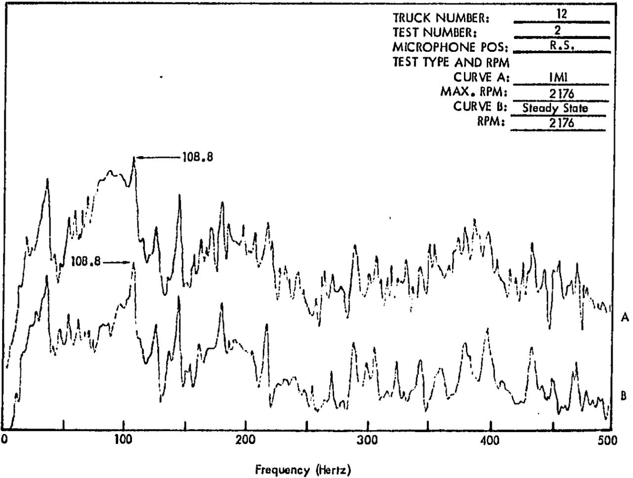
Figure C39. Truck Exterior Noise Spectra (Narrow Band Analysis 1-1/4 Hertz) Measured at 50 Feet. The Spectra Are Used For Determining Engine RPM.
