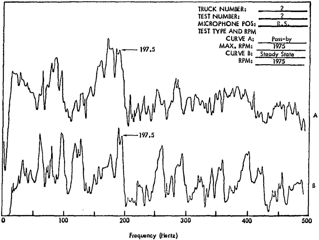
**Figure C6 . Truck Exterior Noise Spectra (Narrow Band Analysis 1-1/4 Hertz) Measured at 50 Feet.
