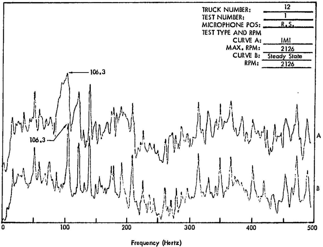
Figure C37. Truck Exterior Noise Spectra (Narrow Band Analysis 1-1/4 Hertz) Measured at 50 Feet. The Spectra Are Used For Determining Engine RPM.
