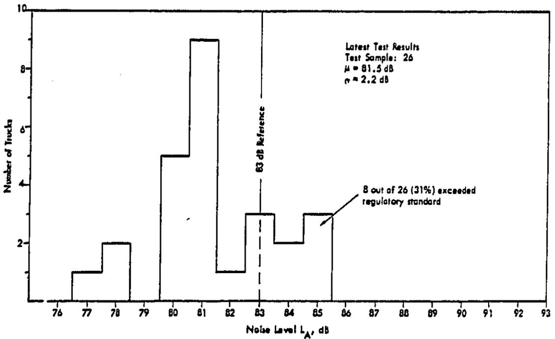
Figure 15. Measured IMI Noise Levels Compared to New Truck Regulations, 83 dB(A)
