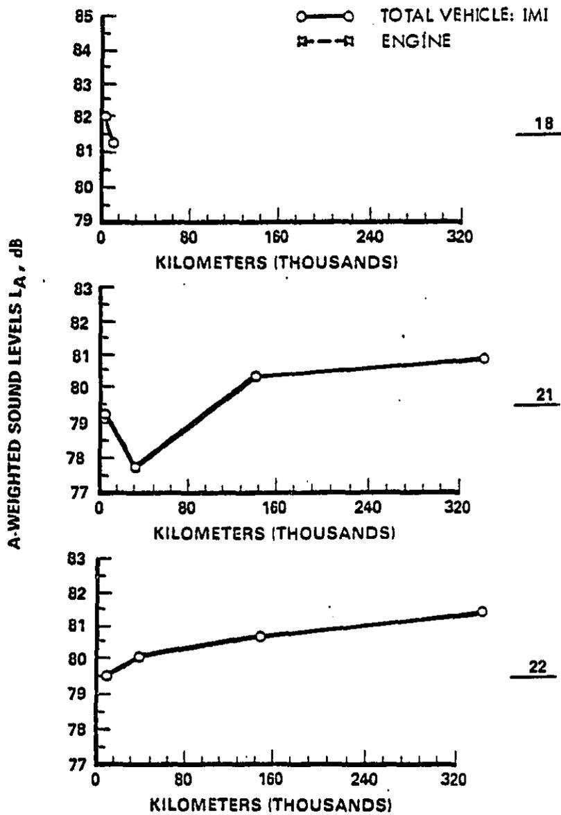
Figure 11. Vehicle Exterior Noise Levels versus Cumulative Kilometers
