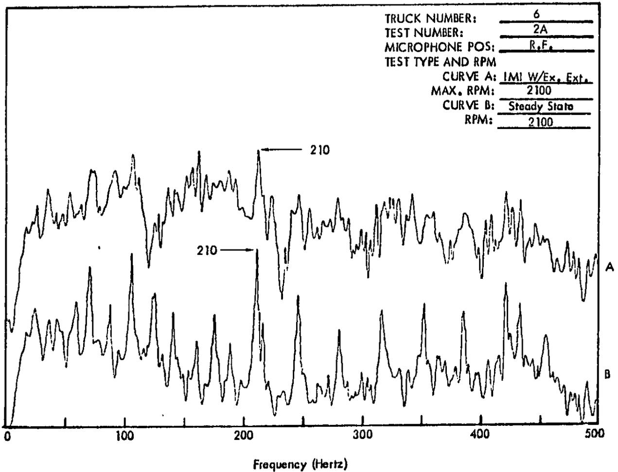
Figure C15. Truck Exterior Noise Spectra (Narrow Band Analysis 1-1/4 Hertz) Measured at 50 Feet.
