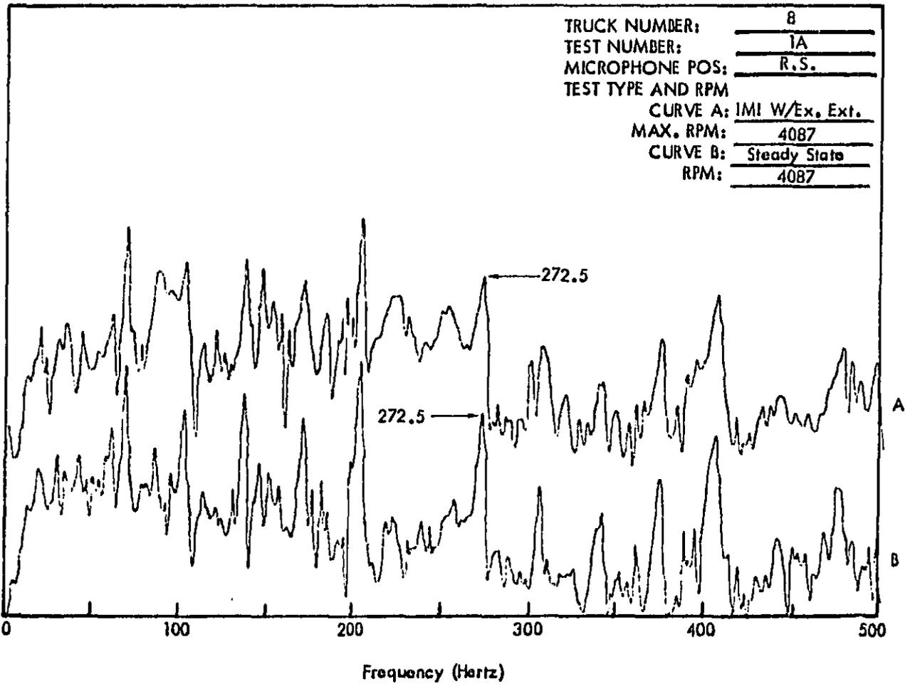
Figure C27 . Truck Exterior Noise Spectra (Narrow Band Analysis 1-1/4 Hertz) Measured at 50 Feet.
