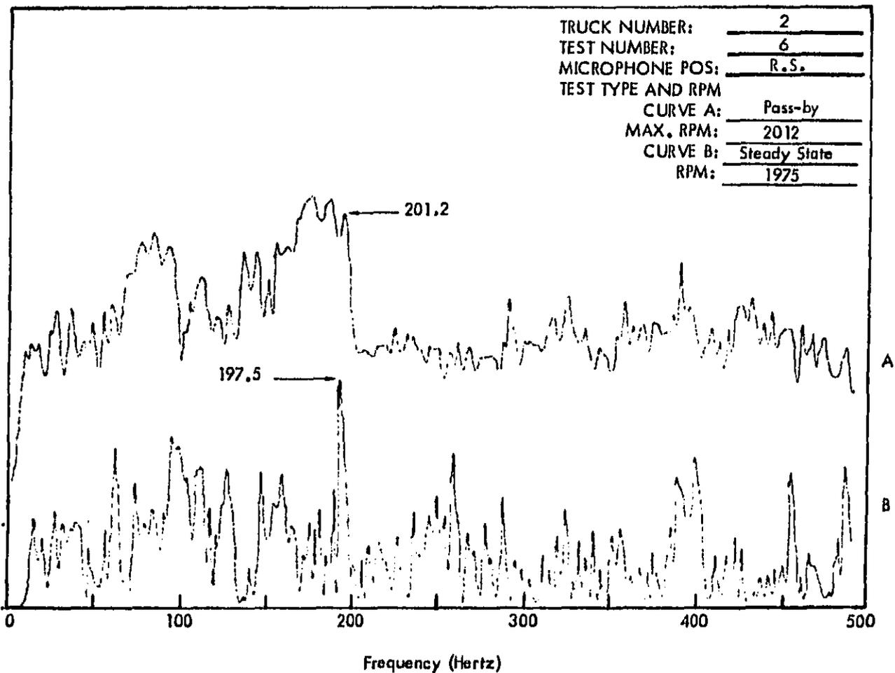
Figure C8 . Truck Exterior Noise Spectra (Narrow Band Analysis 1-1/4 Hertz) Measured at 50 Feet.
