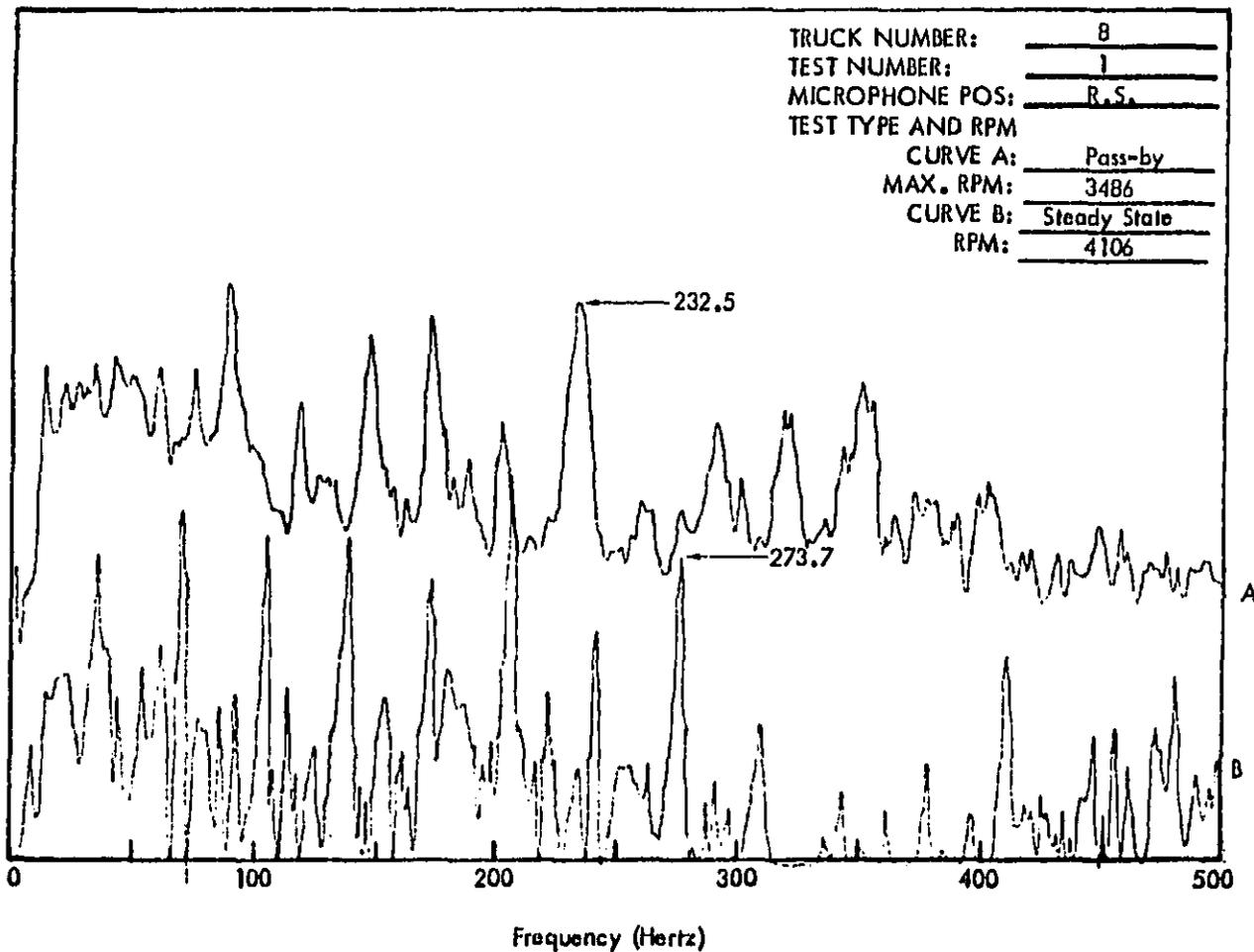
Figure C26 . Truck Exterior Noise Spectra (Narrow Band Analysis 1-1/4 Hertz) Measured at 50 Feet.
