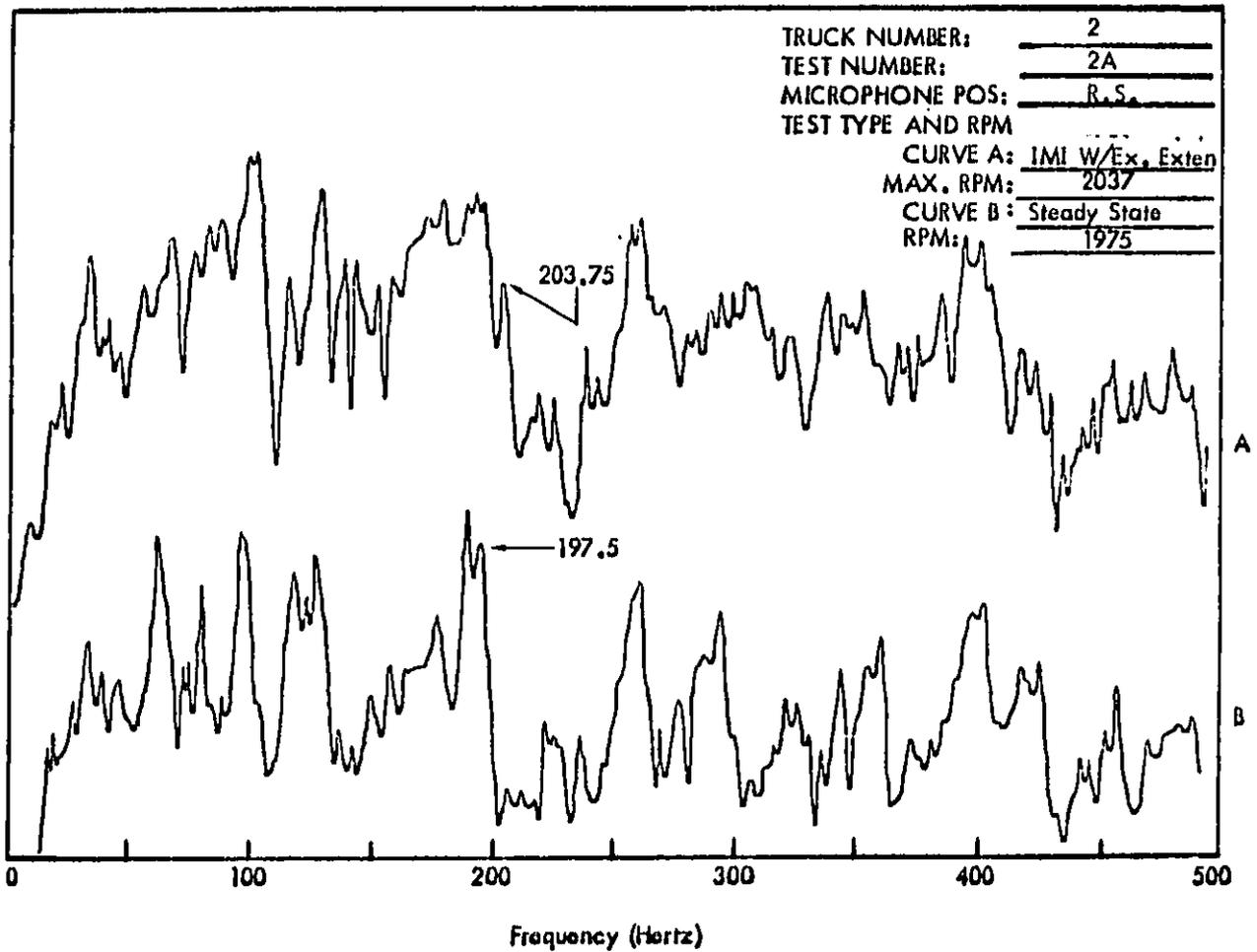
Figure C5 . Truck Exterior Noise Spectra (Narrow Band Analysis 1-1/4 Hertz) Measured at 50 Feet.
