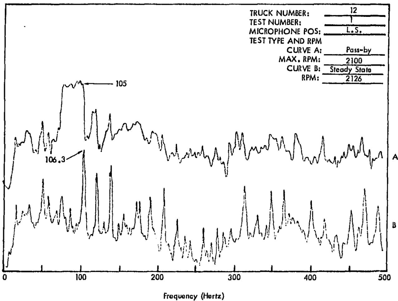
Figure C38 . Truck Exterior Noise Spectra (Narrow Band Analysis 1-1/4 Hertz) Measured at 50 Feet.
