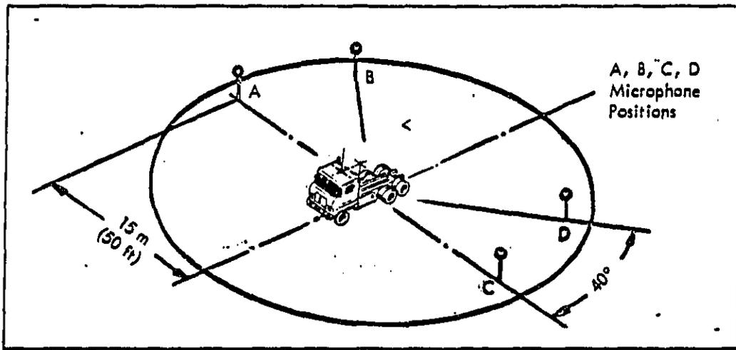
Figure 4. Microphone Positions for Stationary Testing
