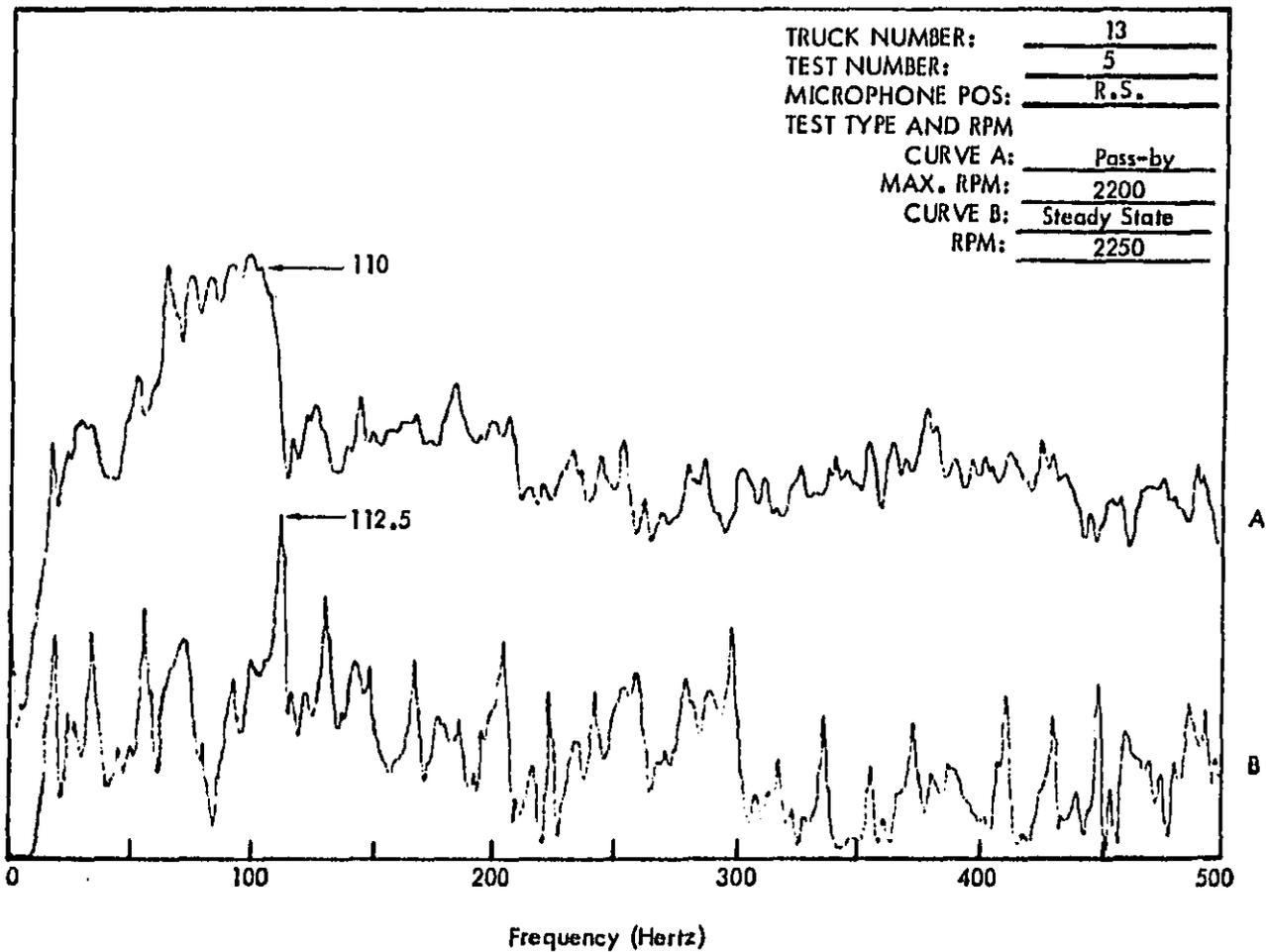
Figure C47 . Truck Exterior Noise Spectra (Narrow Band Analysis 1-1/4 Hertz) Measured at 50 Feet.
