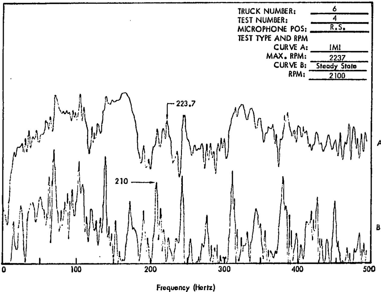
Figure C16 . Truck Exterior Noise Spectra (Narrow Band Analysis 1-1/4 Hertz) Measured at 50 Feet.
