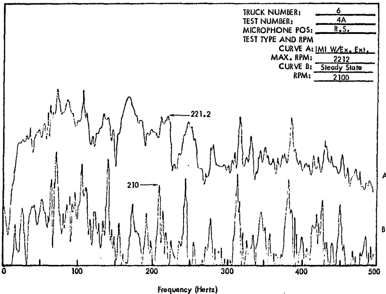
Figure C18. Truck Exterior Noise Spectra (Narrow Band Analysis 1-1/4 Hertz) Measured at 50 Feet.
