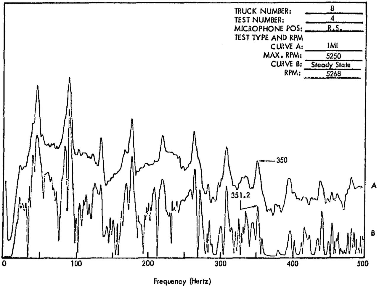
Figure C28. Truck Exterior Noise Spectra (Narrow Band Analysis 1-1/4 Hertz) Measured at 50 Feet.
