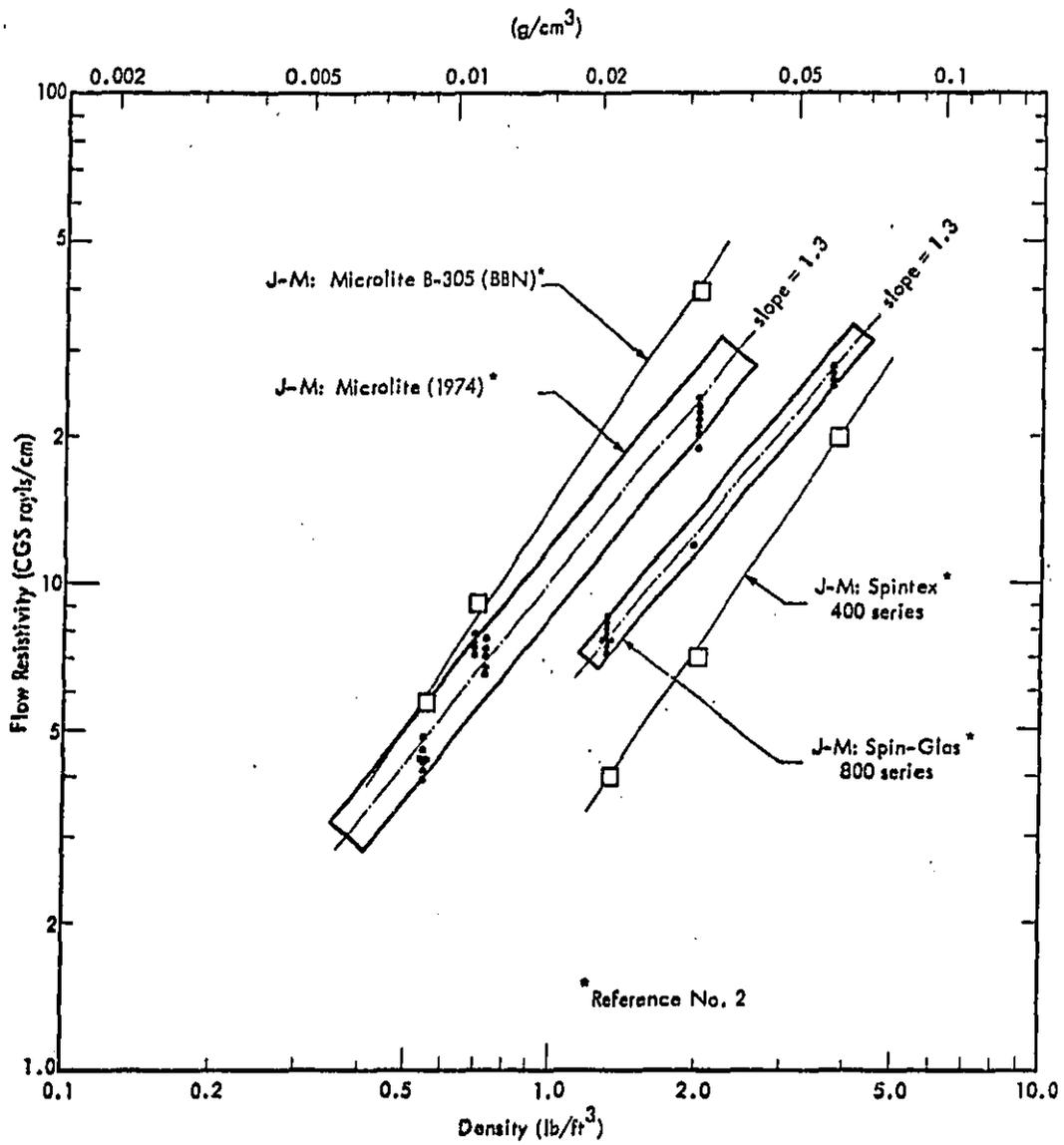
Figure 2. Flow Resistivity Apparatus Verification
