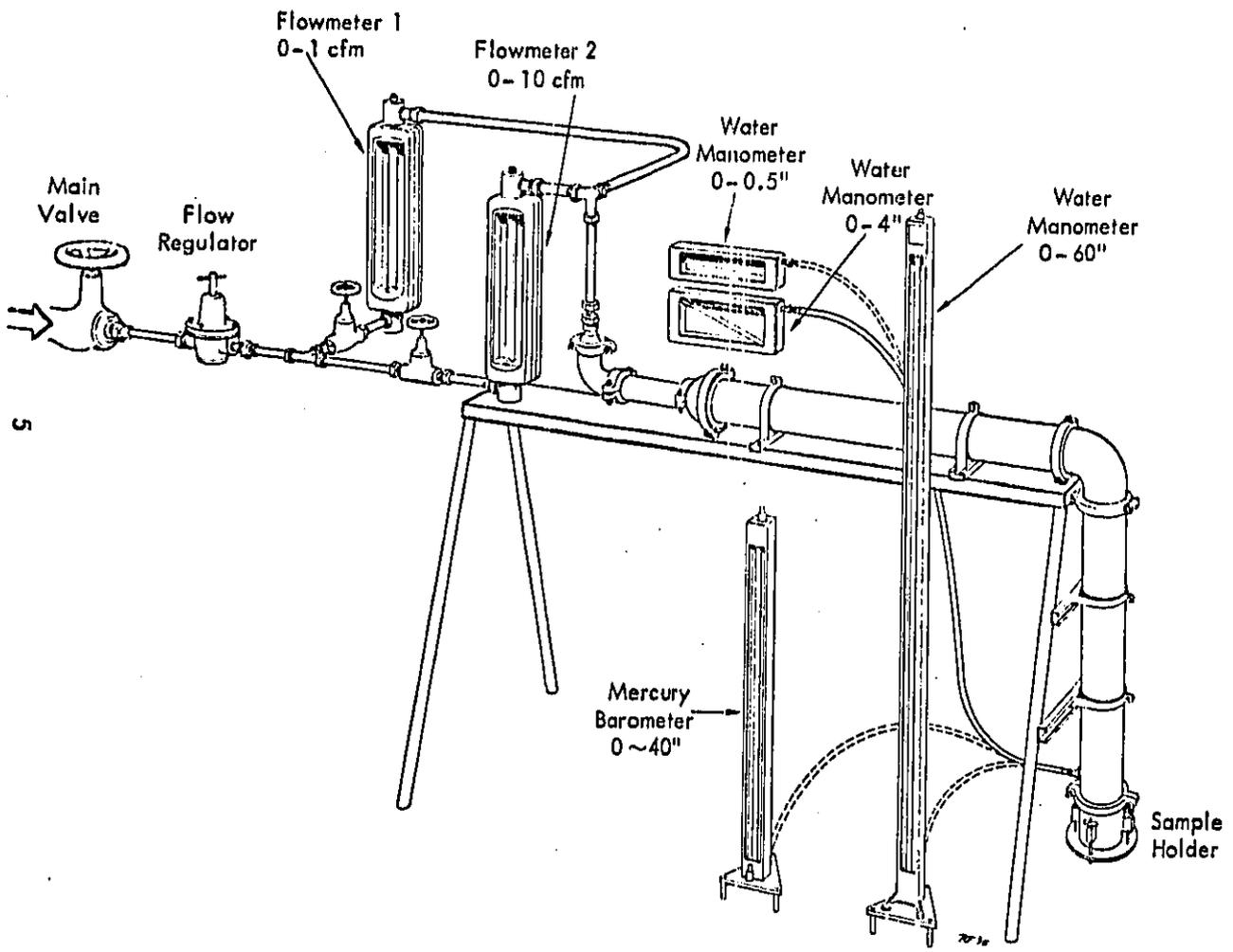
Figure 1. Flow Resistivity Apparatus
