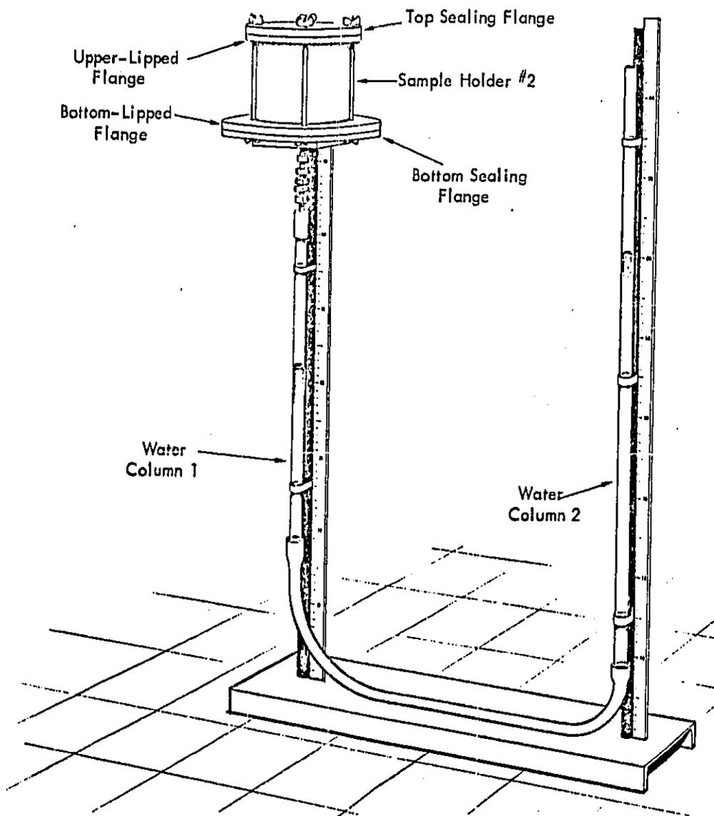
Figure 4. Porosity Measurement Apparatus
