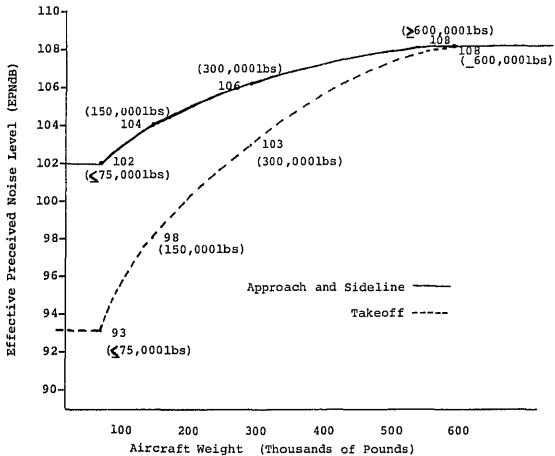
Many other factors such as weight of the aircraft, configuration of the flaps, and glide path are specified for the purposes of the testing. Note in the chart that two sideline measuring distances are shown. The .25 NMi distance applies to aircraft of less than four engines and the .35 NMi for the four or more engine category.
