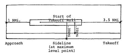
Using these measuring points, the aircraft type must be capable of limiting the noise generated according to the following graph:
