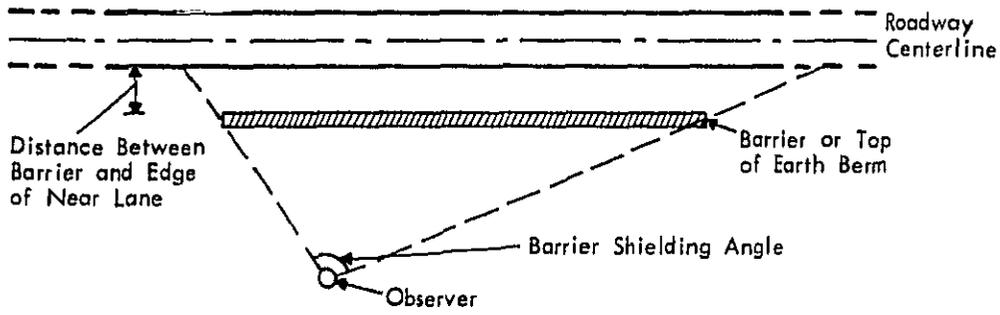
A. Barrier Shielding Parameters
