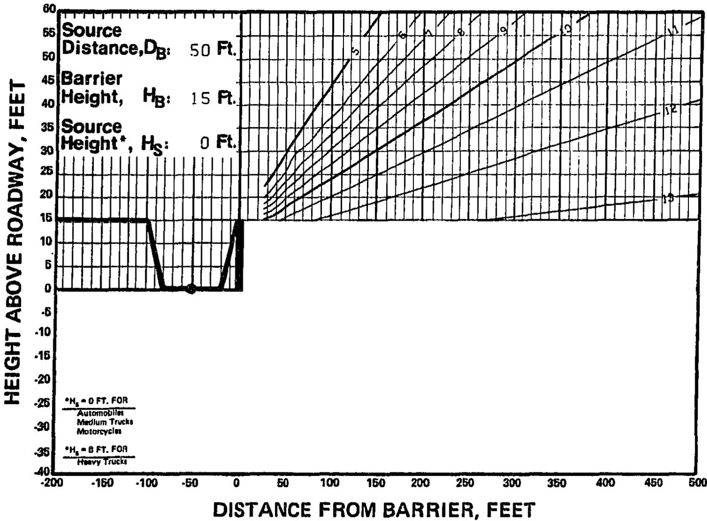
FIGURE 5-3. USE OF BARRIER ATTENUATION CHART FOR DEPRESSED ROADWAYS
