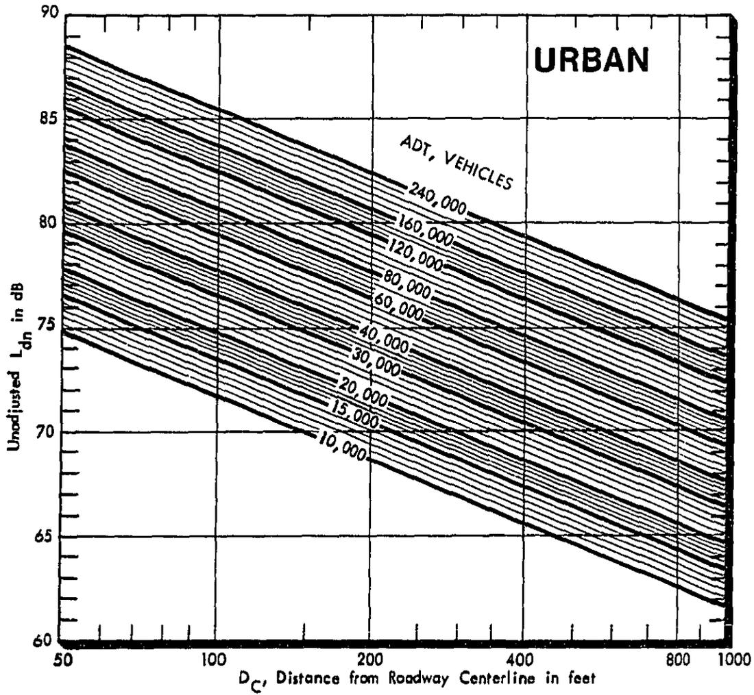
FIGURE 3-2A. CHART FOR ESTIMATING UNADJUSTED  $L_{dn}$  FOR URBAN AREAS
