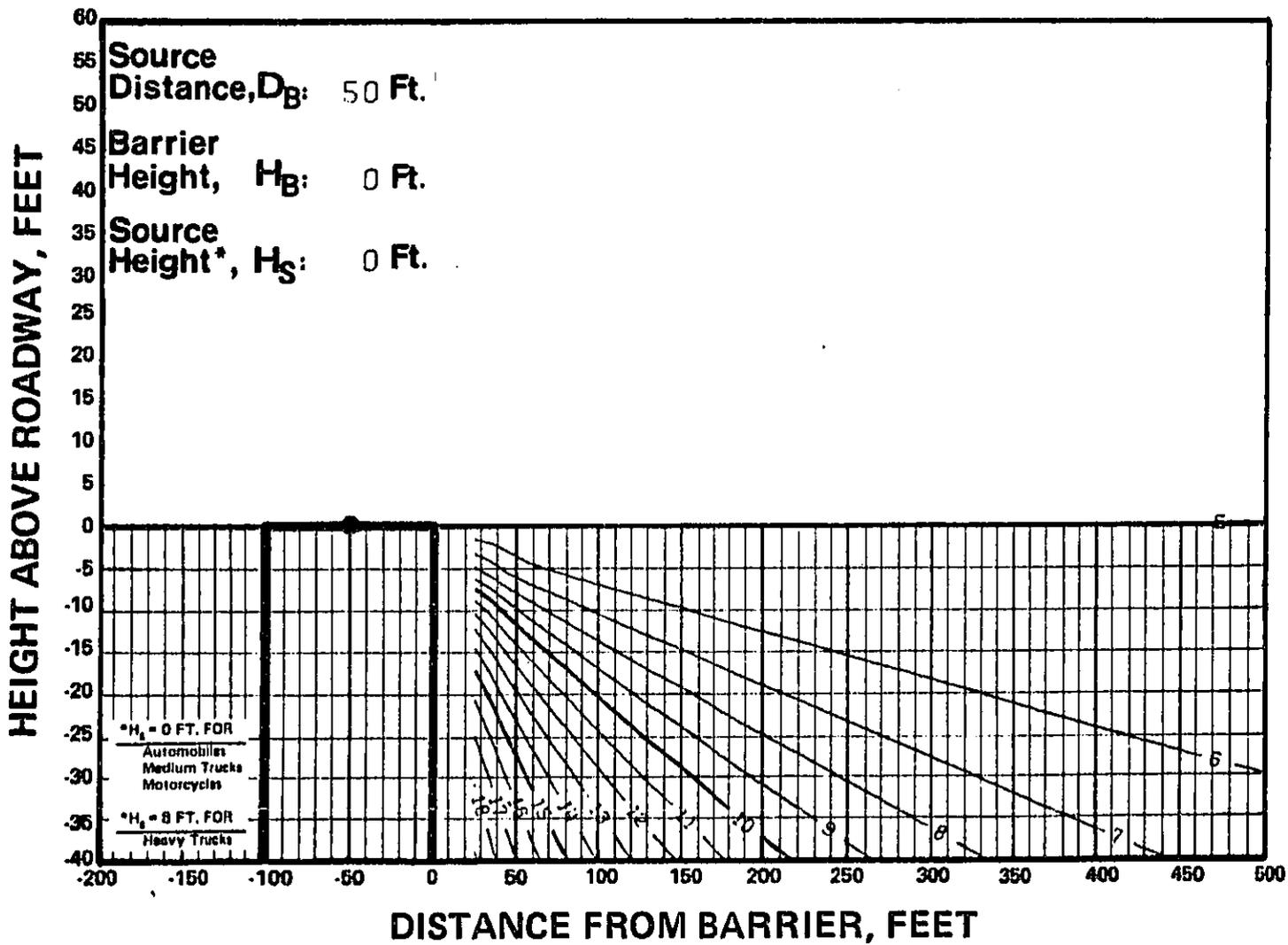
FIGURE 5-2. USE OF BARRIER ATTENUATION CHART FOR ELEVATED ROADWAYS
