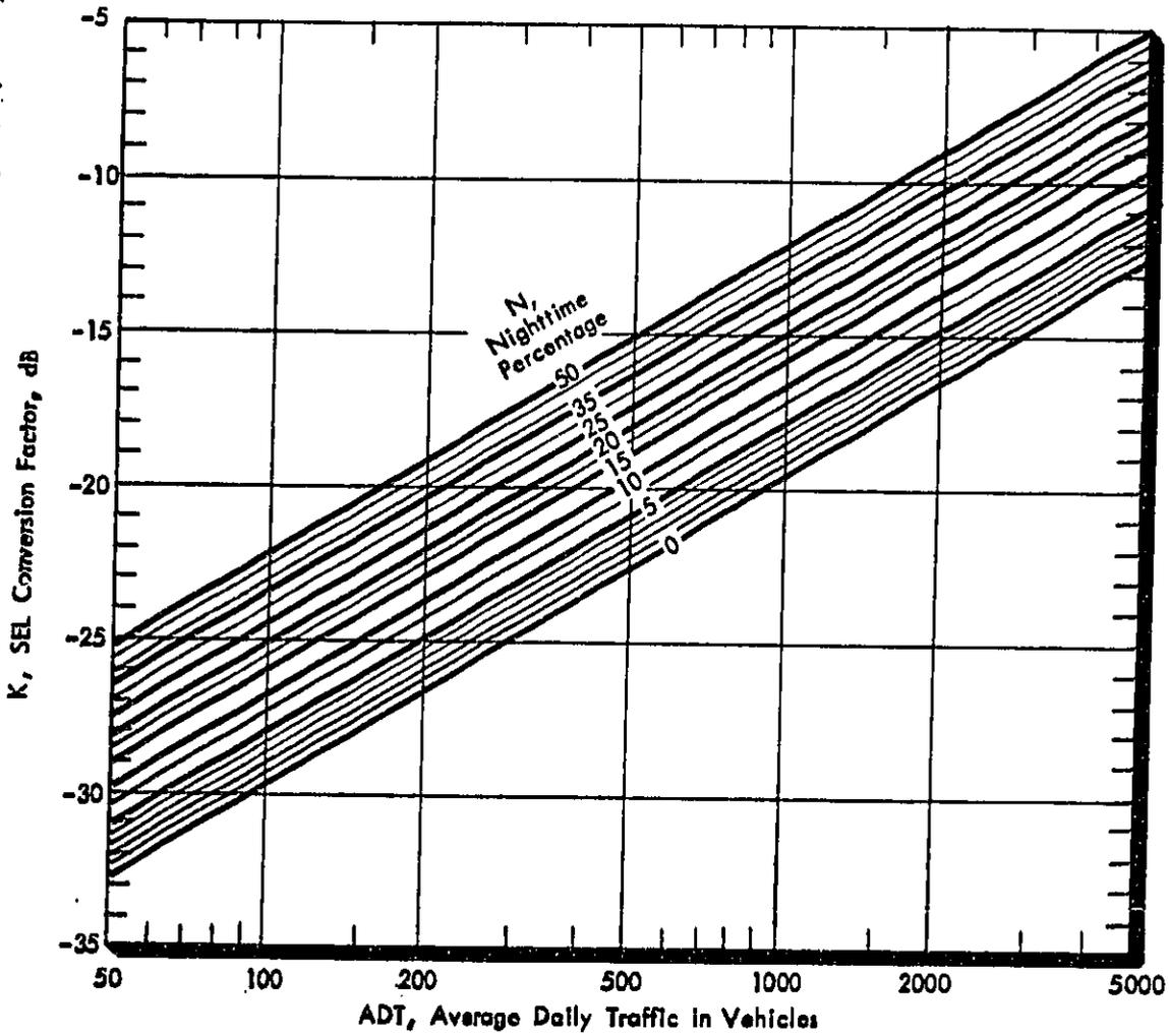
FIGURE 4-8B. CONVERSION FACTOR FOR SEL TO  $L_{dn}$
