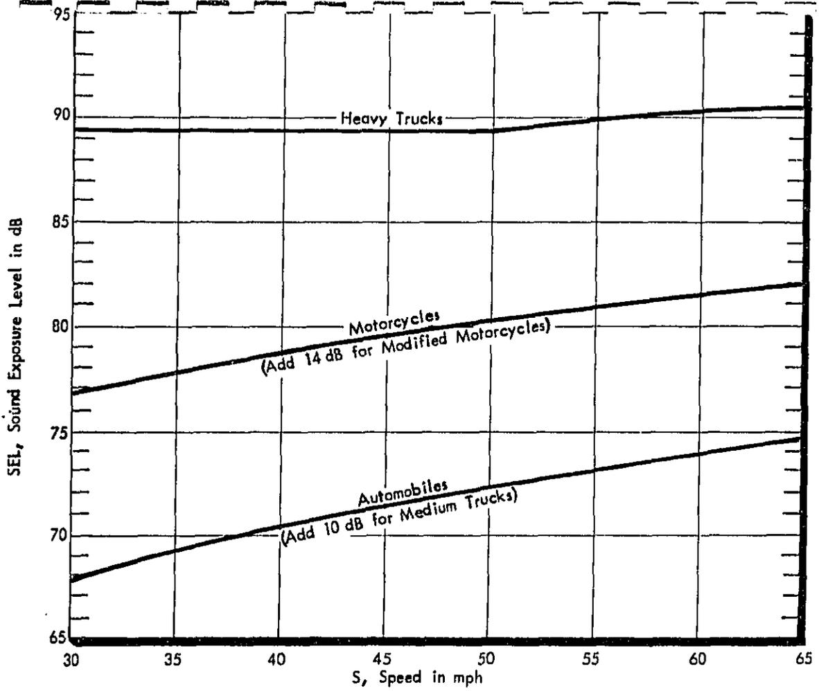
FIGURE 4-5. VEHICLE SOUND EXPOSURE LEVELS AT 50 FEET
