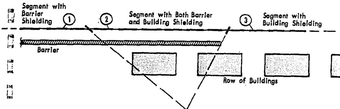
D. ROADWAY WITH MULTIPLE SHIELDING ELEMENTS (PLAN VIEW)
