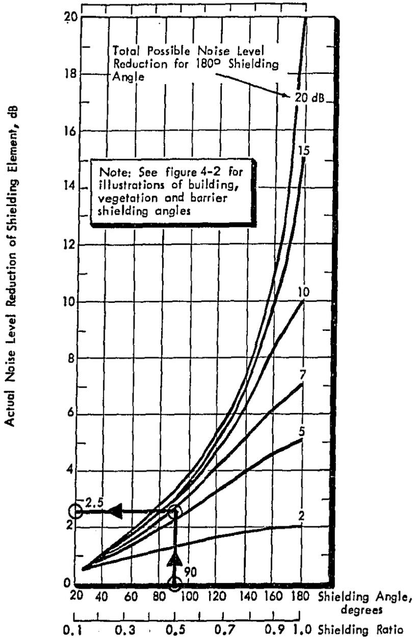
ILLUSTRATION 4-8. USE OF SHIELDING ELEMENT ADJUSTMENT CHART
