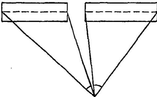
SEGMENT ANGLE FOR SEGMENTS WITH DEFINITE ENDS
