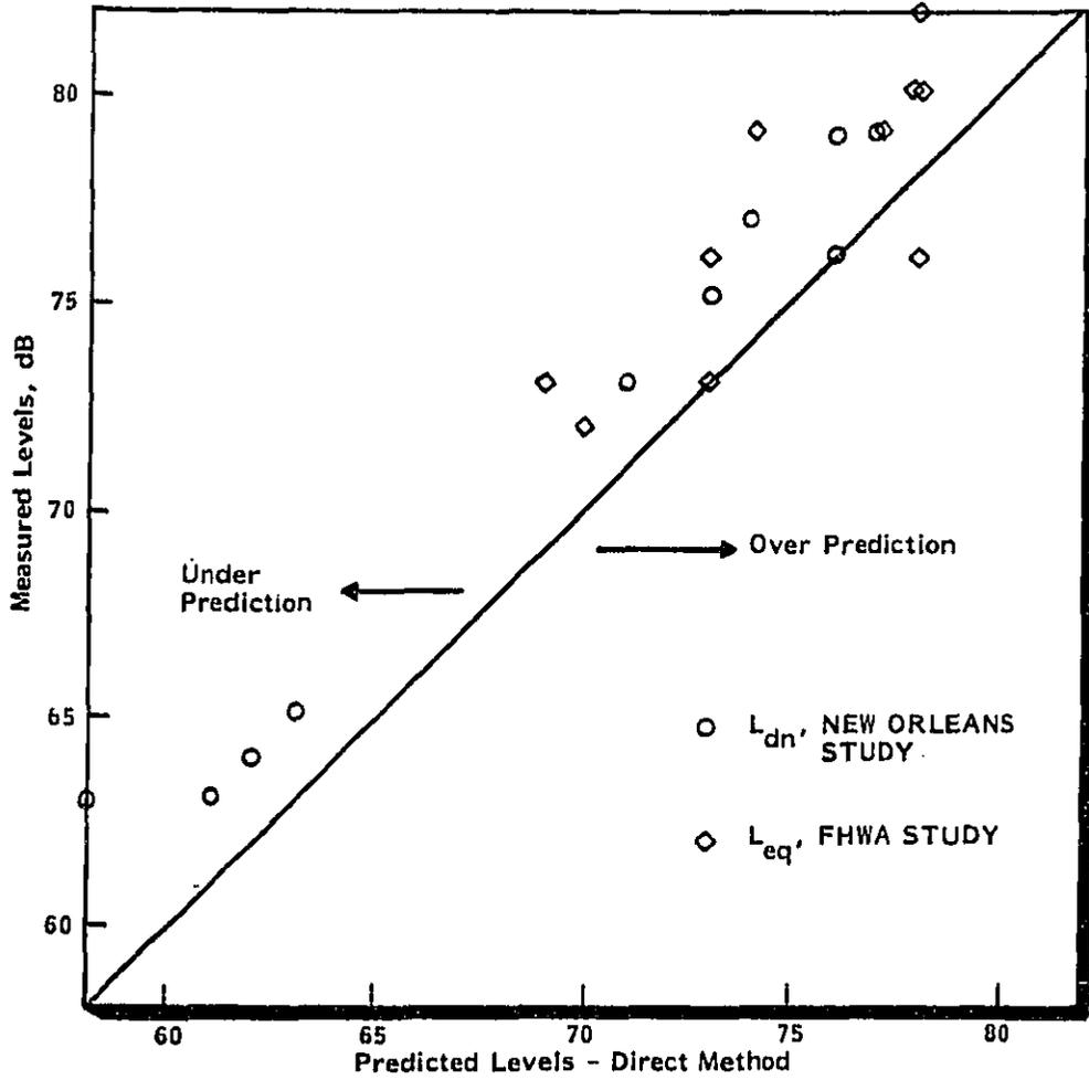
FIGURE E-3. MEASURED VS. PREDICTED LEVELS USING THE DIRECT METHOD
