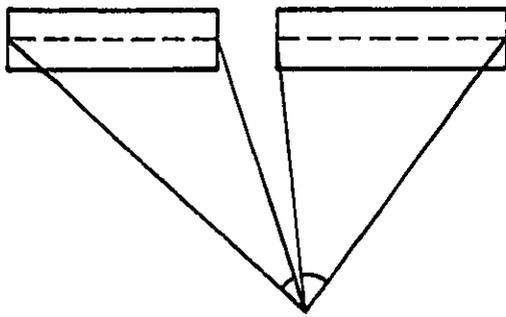
SEGMENT ANGLE FOR SEGMENTS WITH DEFINITE ENDS
