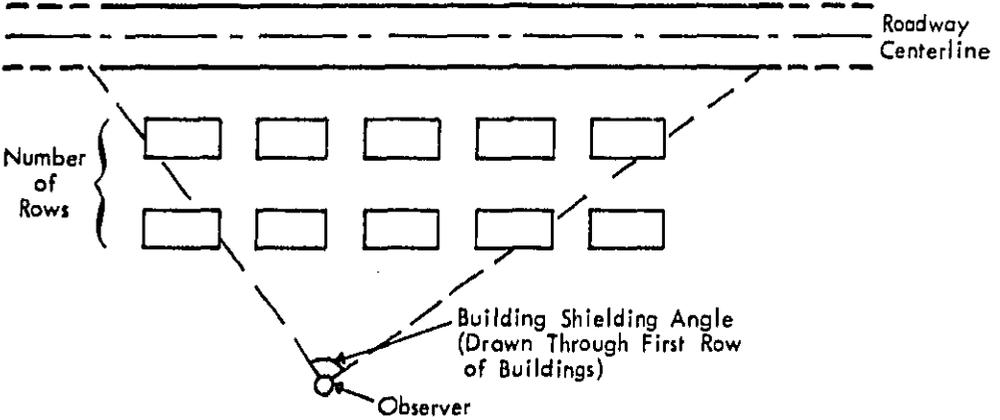
B. Building Shielding Parameters
