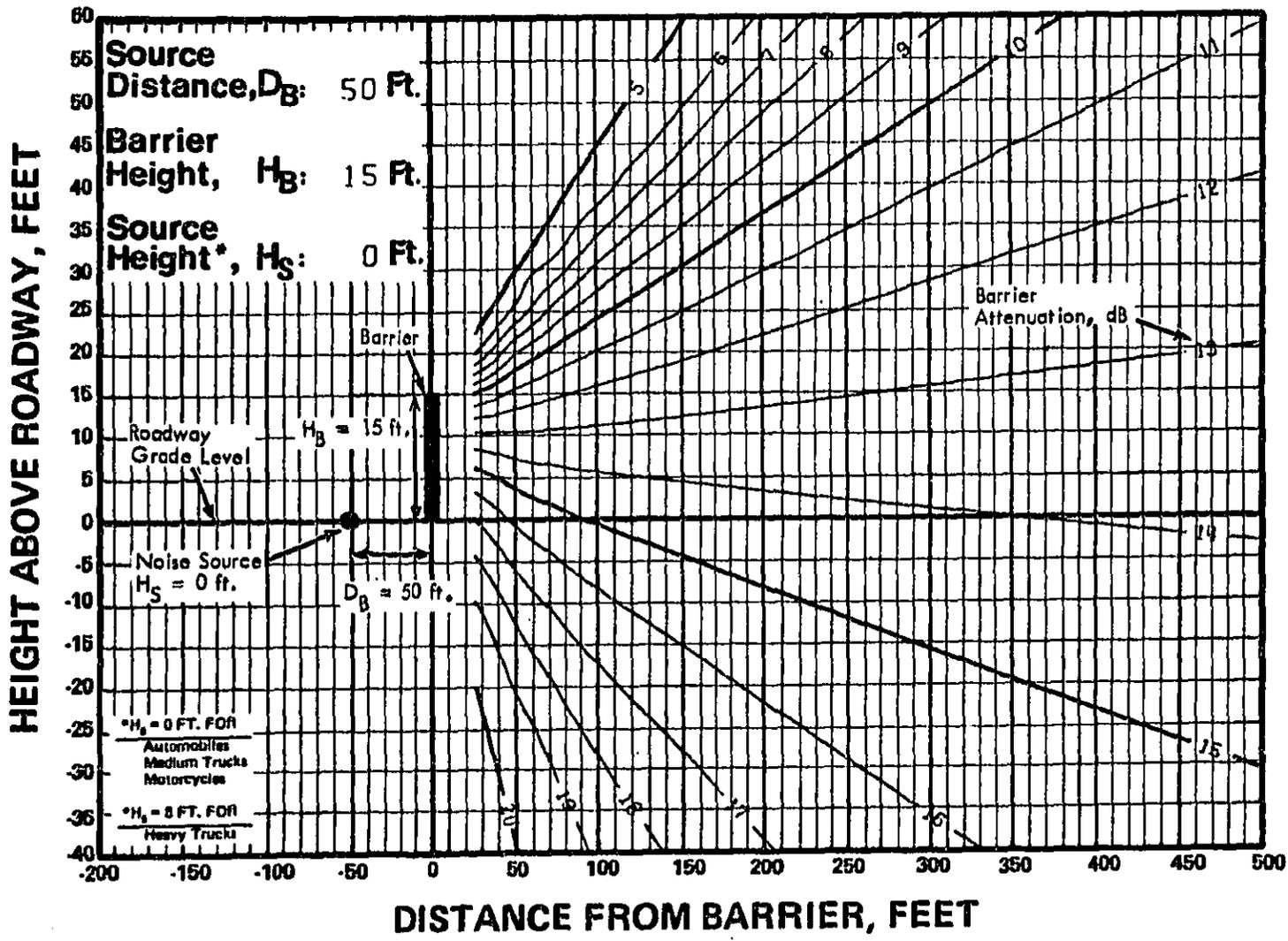
FIGURE 4-13. SAMPLE BARRIER ATTENUATION CHART
