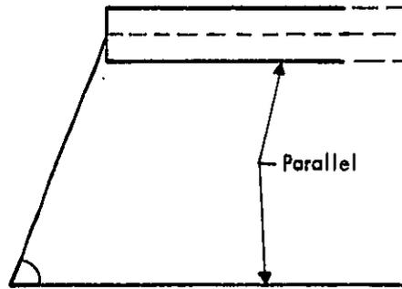
SEGMENT ANGLE FOR SEGMENTS WITH INDEFINITE ENDS
