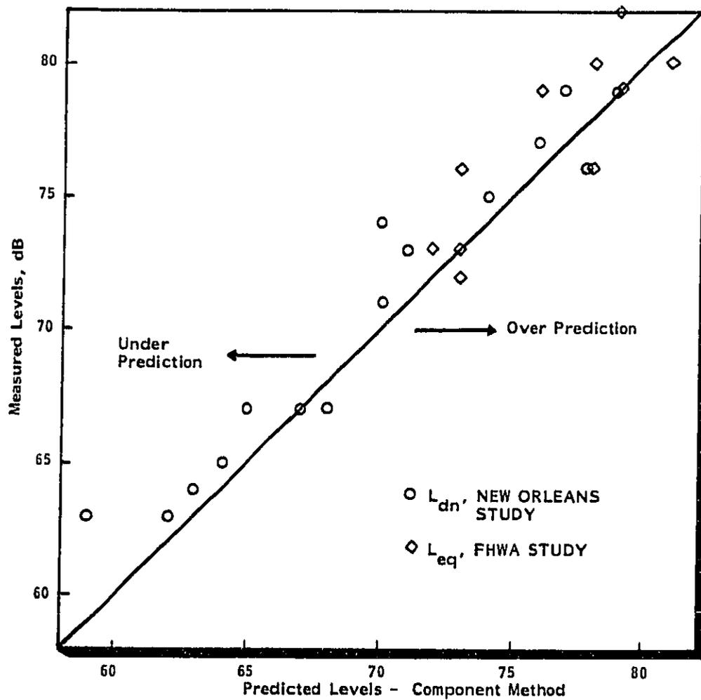
FIGURE E-4. MEASURED VS. PREDICTED LEVELS USING THE COMPONENT METHOD
