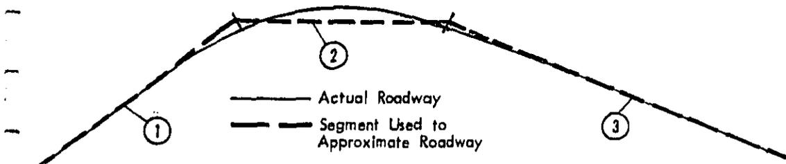
A. ROADWAY WITH CURVED ALIGNMENT (PLAN VIEW)
