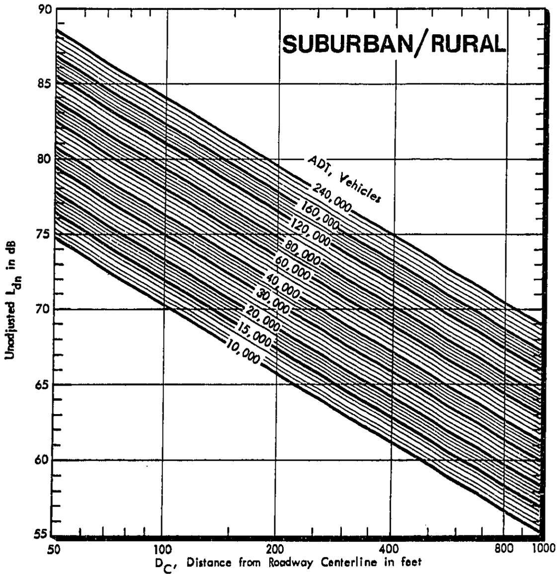
FIGURE 3-2B. CHART FOR ESTIMATING UNADJUSTED  $L_{dn}$  FOR SUBURBAN AND RURAL AREAS
