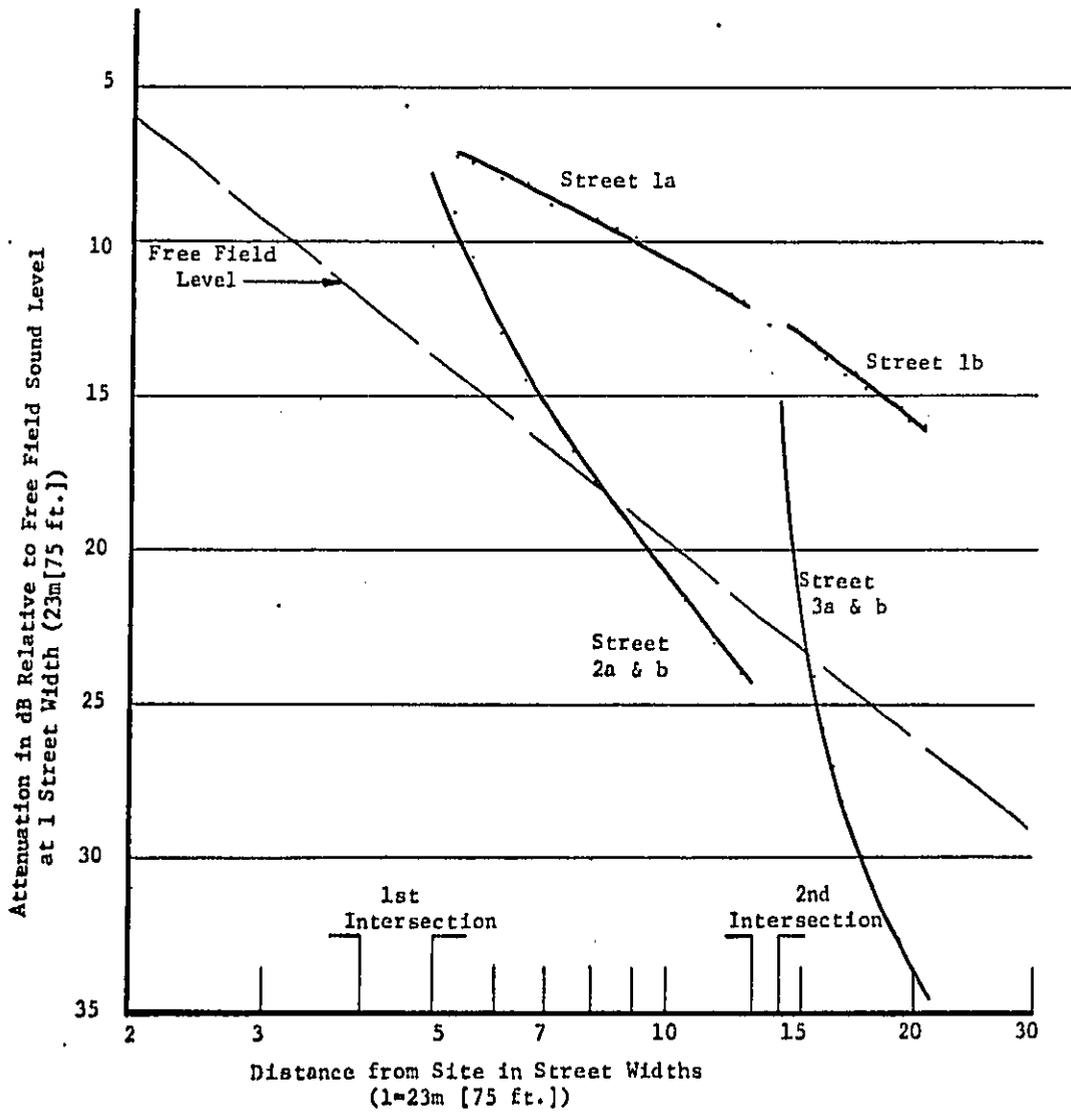
Figure 10: Attenuation as a Function of Distance for Case I, Site A
