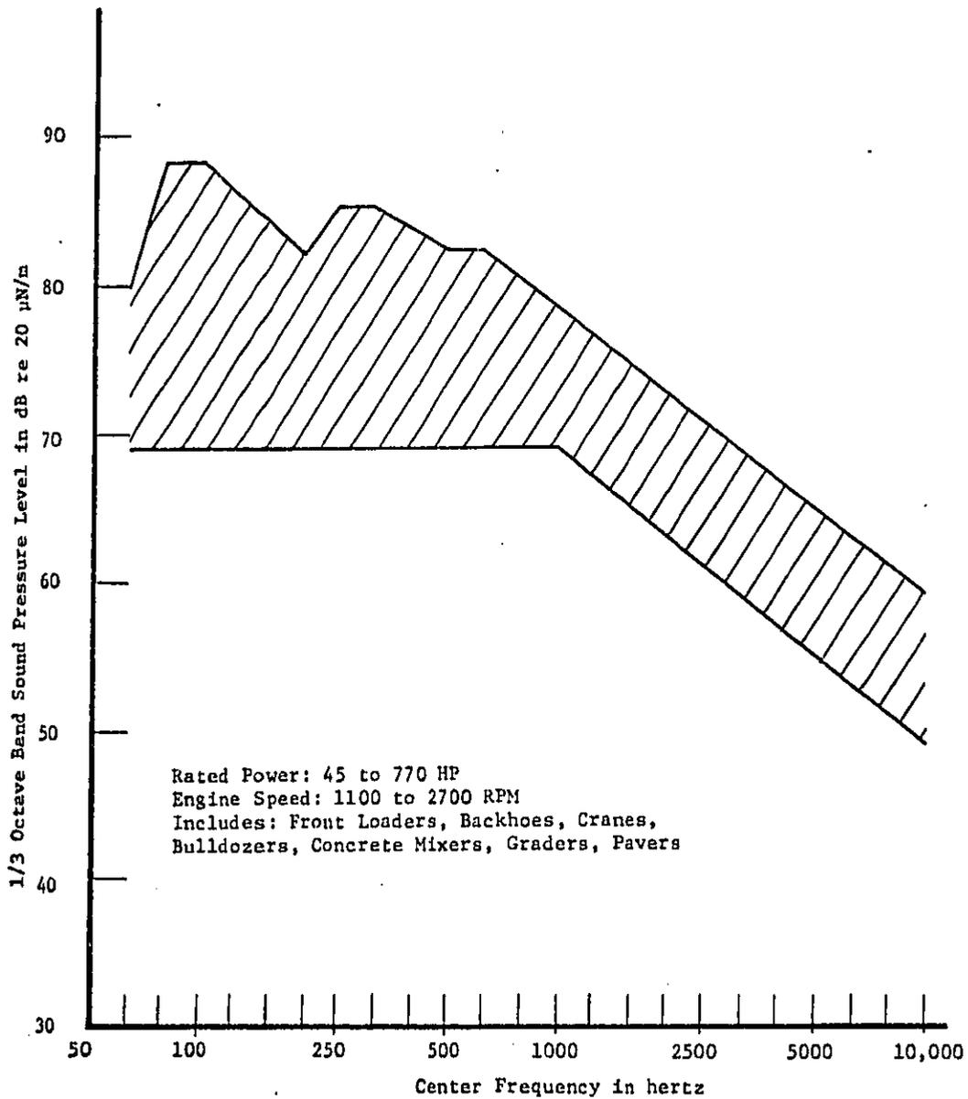
Figure 9: Envelope of Sound Pressure Levels from 23 Diesel-powered Items of Construction Equipment as Measured at 15m (50 ft)
