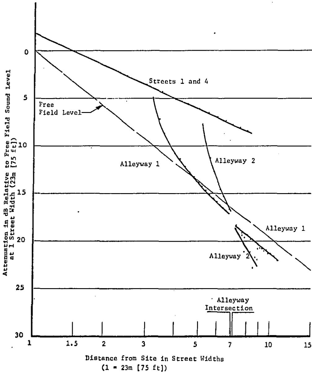
Figure 19: Attenuation as a Function of Distance for Case II, Site A, Alleyways 1 and 2 (strictly valid for only octave band sound pressure levels greater than 500 Hz.)
