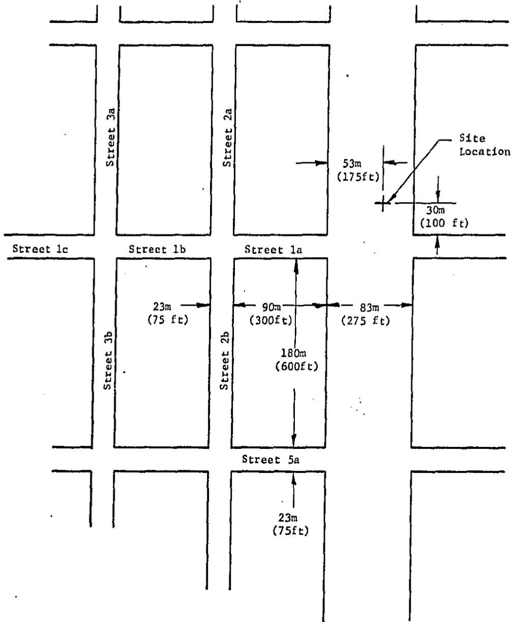
Figure 8: Assumed Geometry for Computed Attenuation Values for Block Configuration Case II, Site B
