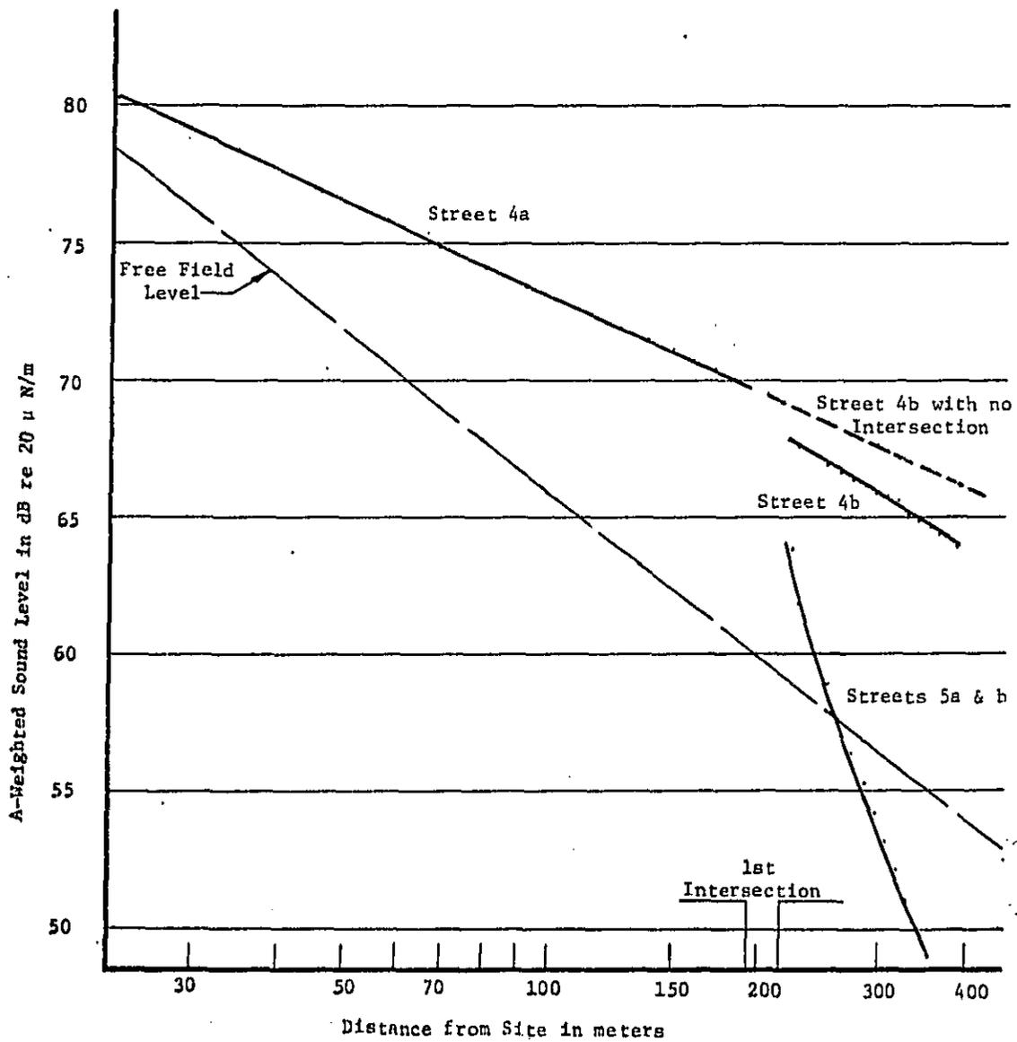
Figure 17: A-Weighted Sound Levels as a Function of Distance for Case II, Site A, Streets 4 and 5 for a Source Level of 82 dB at 15m (50 ft)
