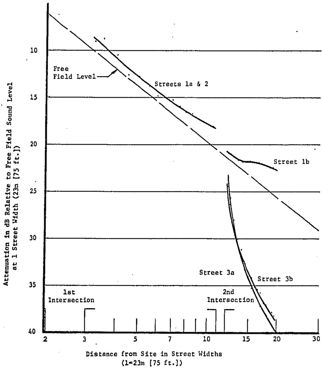
Figure 11: Attenuation as a Function of Distance for Case I, Site B
