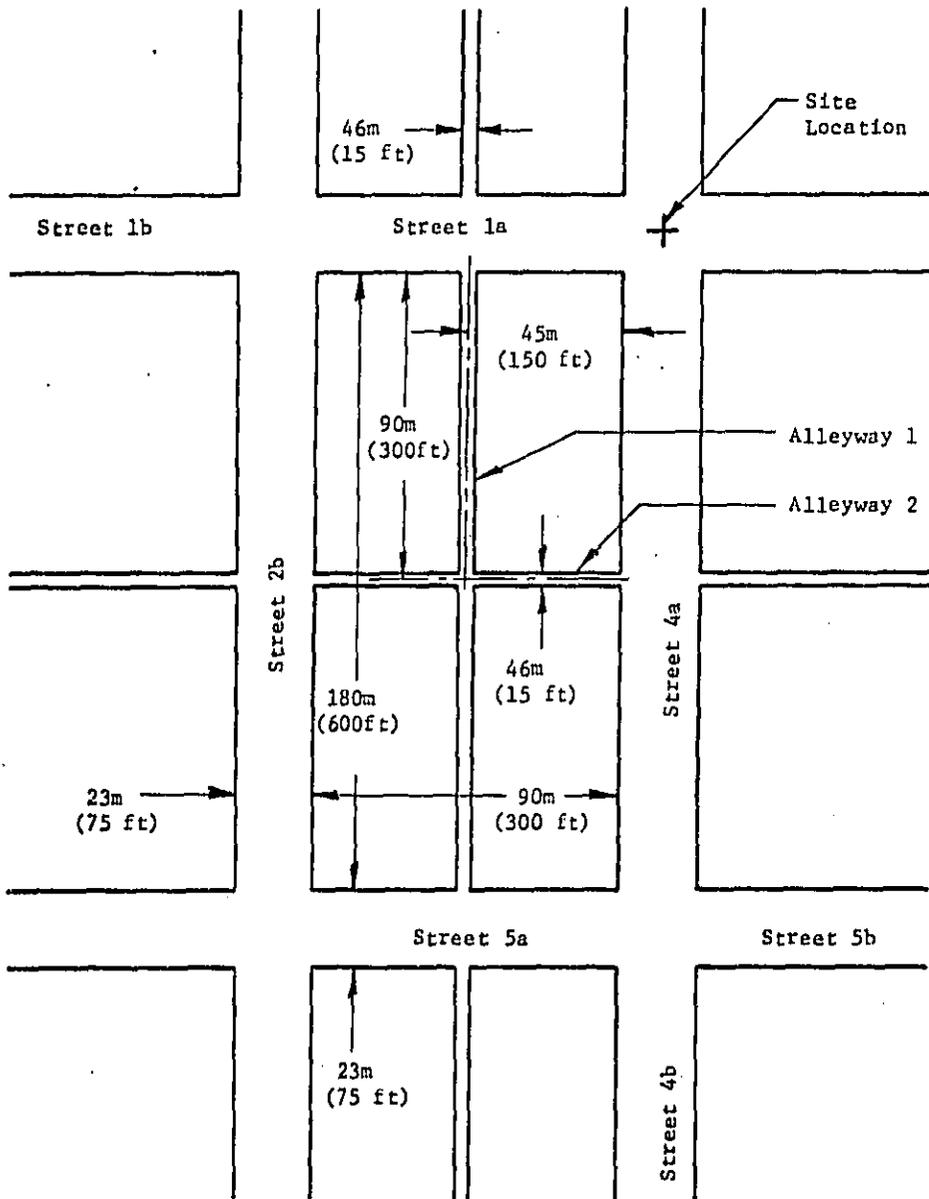
Figure 18: Geometry and Nomenclature for Assessment of Sound Propagation into Blocks Along Alleyways - Case II, Site A
