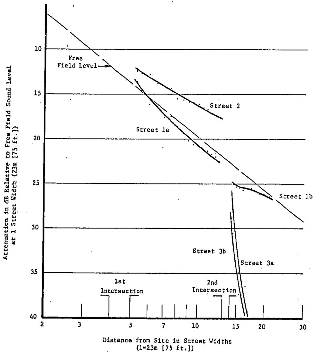
Figure 12: Attenuation as a Function at Distance for Case I, Site C.
