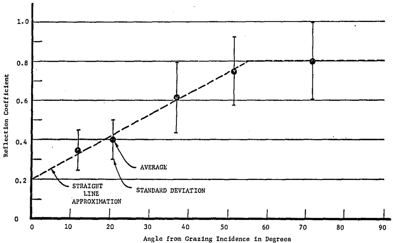
Figure 1: Measured Reflection Coefficients with Two Segment Linear Approximation Averaged for Frequencies Corresponding to 250, 500, 1000, 2000 hertz (From Reference 11)
