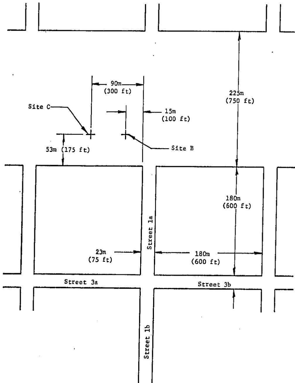
Figure 7: Assumed Geometry for Computed Attenuation Values for Block Configuration Case I, Sites B and C.
