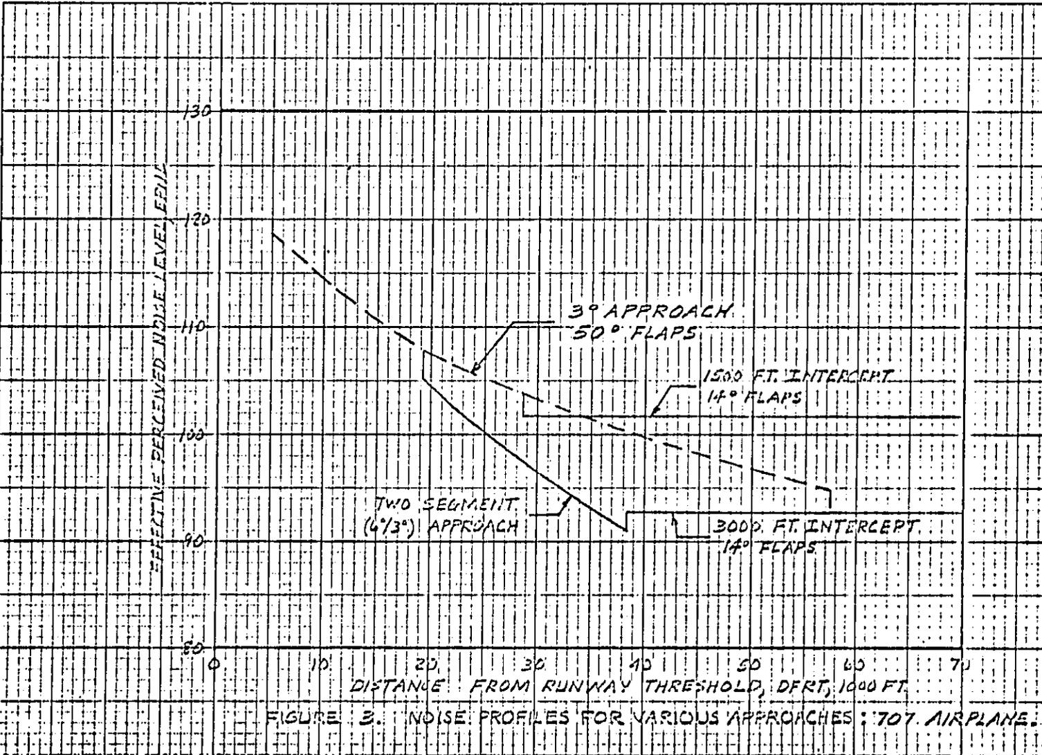
FIGURE 3. NOISE PROFILES FOR VARIOUS APPROACHES: 707 AIRPLANE.
