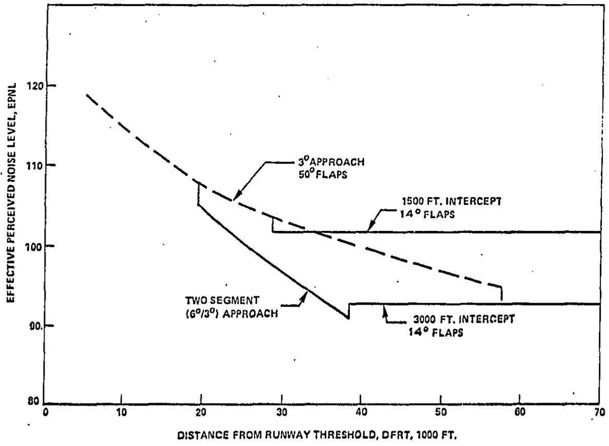
FIGURE 2. NOISE PROFILES FOR VARIOUS APPROACHES: 707 AIRPLANE
