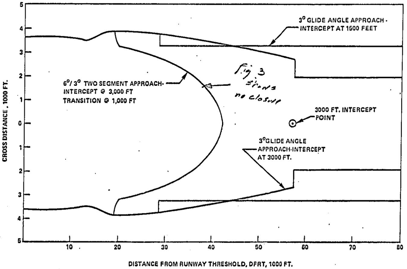
FIGURE 3. 90 EPndB CONTOURS FOR VARIOUS APPROACHES: 707 AIRPLANE
