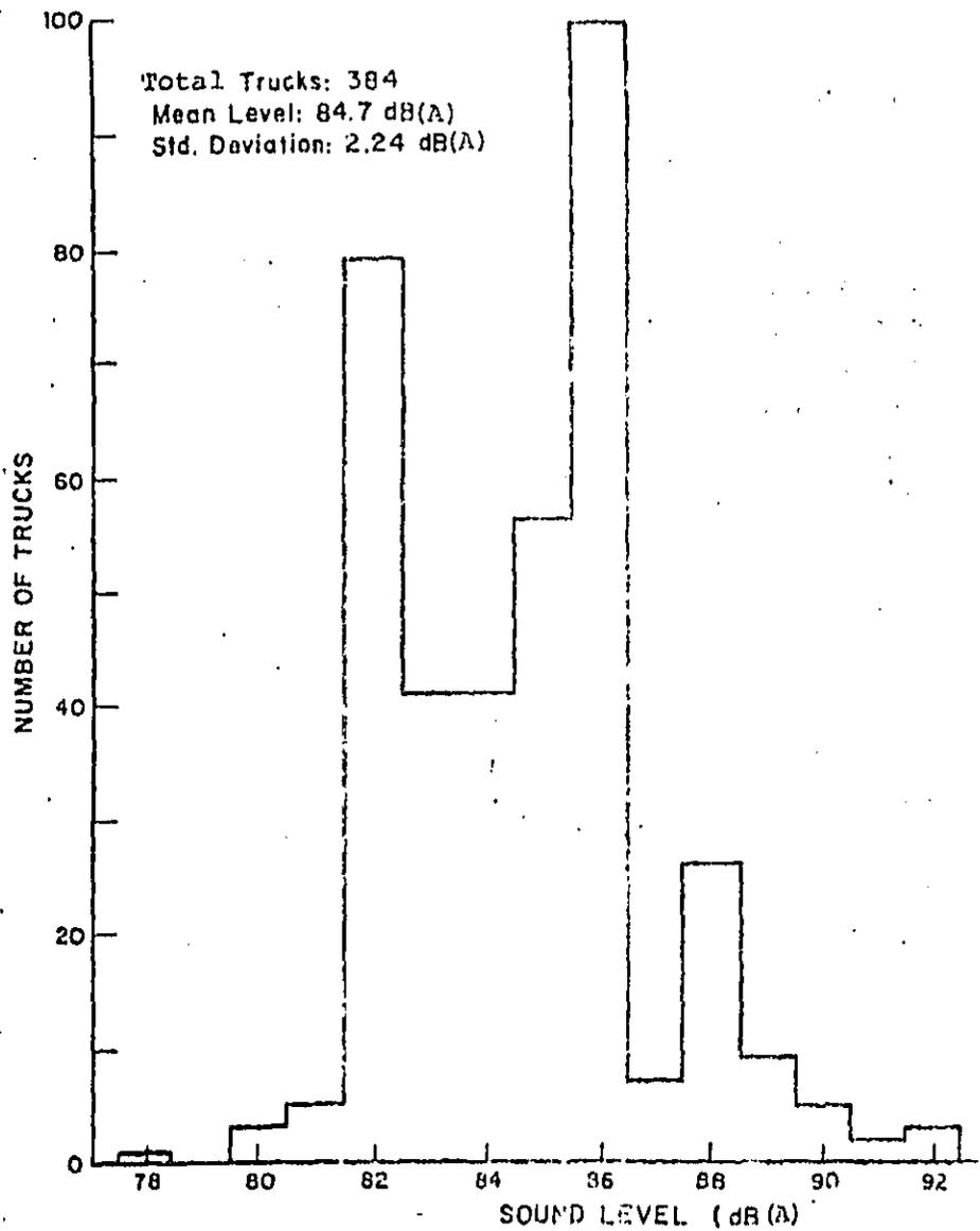
Figure 4-2 Histogram of New Diesel Truck Noise Levels.
