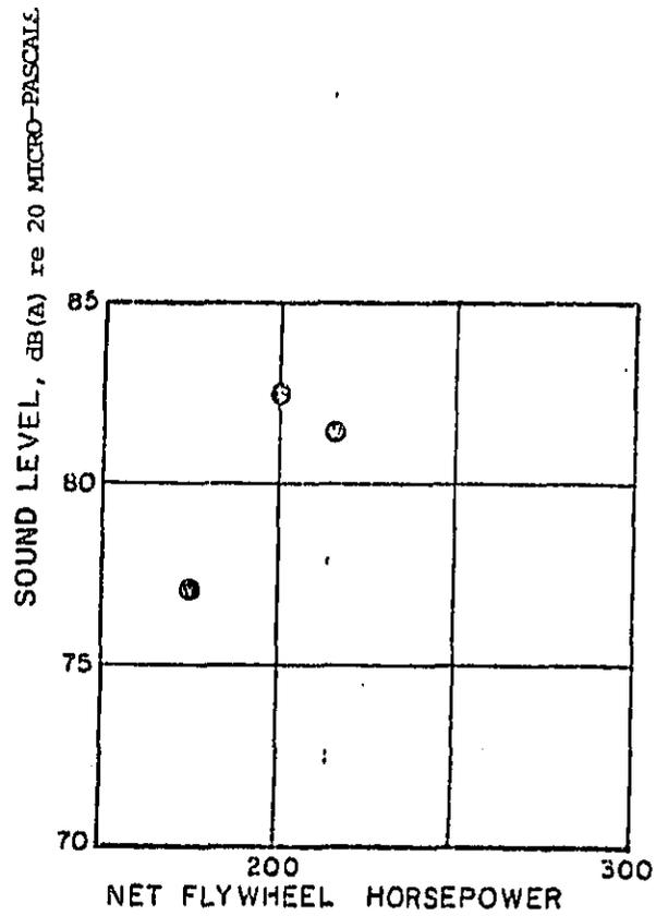
Figure 5-4 Gasoline-Fueled Truck Fan Noise Levels as a Function of Engine Horsepower.
