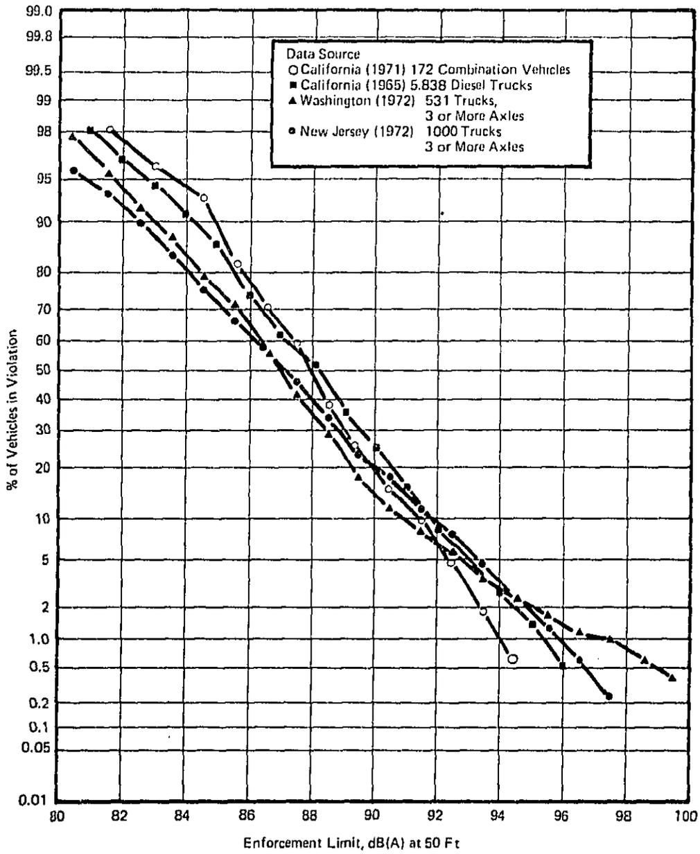
Figure 10. Enforcement Limit, dB(A) At 50 Ft
