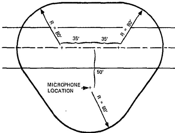
Figure A-1. Test site clearance requirements for pass-by test.
