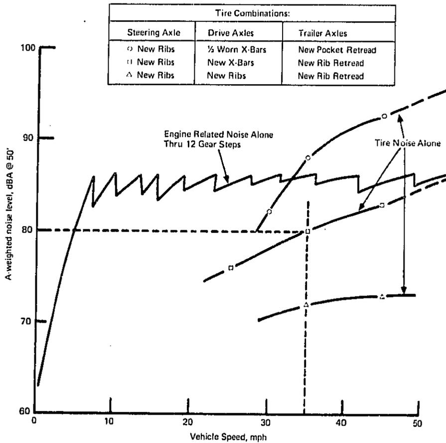
Figure 2. Propulsion System and Tire Noise for a Typical 5 Axle Tractor Trailer (from reference 6 and 7)
