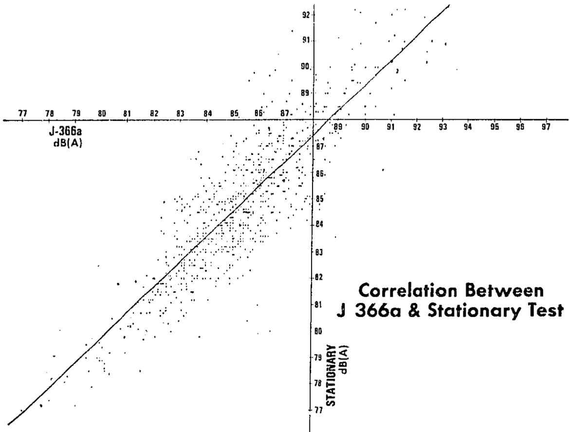
Figure 8. Plot of Test Results According to SRUT and SAE J366a for 877 Trucks.
