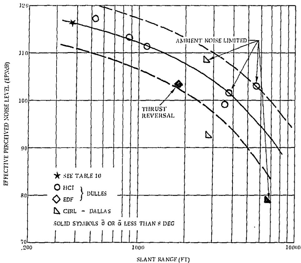
Figure 14. EPNL Versus Slant Range Approach
