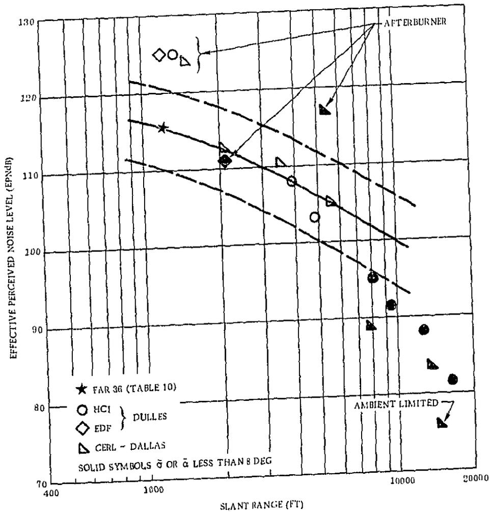
Figure 12. EPNL Versus Slant Range Takeoff
