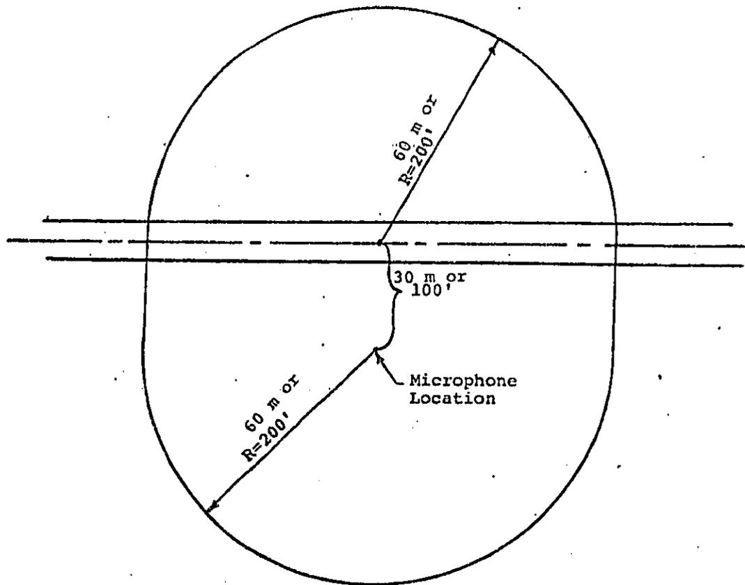
Figure 6-2. Test Site Clearance Requirement for Locomotive Stationary Test
