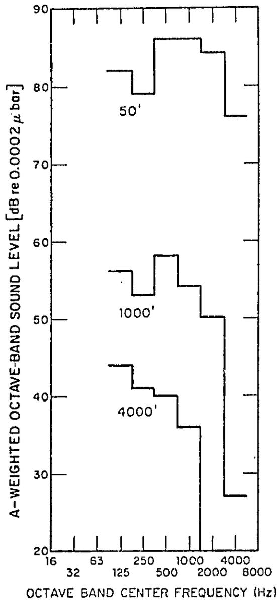
Figure 8-7. Influence of Frequency-Dependent Attenuations on Locomotive Noise Spectrum
