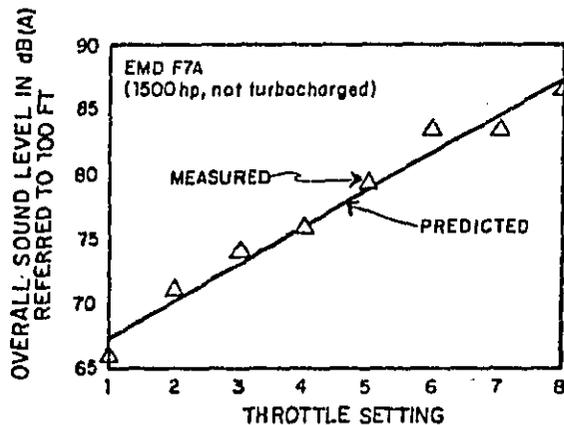
Figure 4-1. Measured Total and Predicted Exhaust Noise Levels
