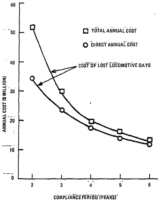
Figure 7-1. Cost of Retrofit Program as a Function of Compliance Period
