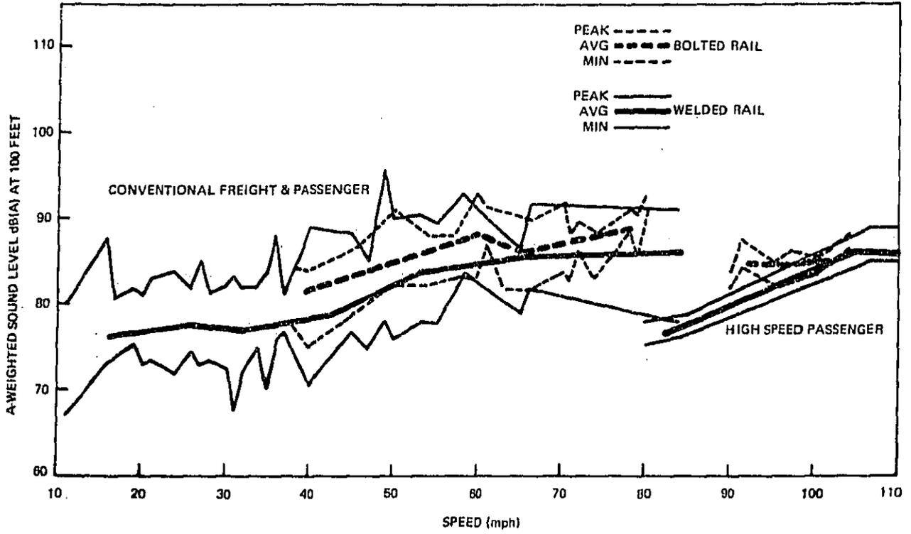
Figure 4-8. Average, and Minimum Rail-Wheel Sound Level vs. Speed for Typical Railroad Cars on Welded and Bolted Rail
