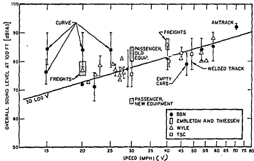
Figure 4-7. Measured Wheel/Rail Noise
