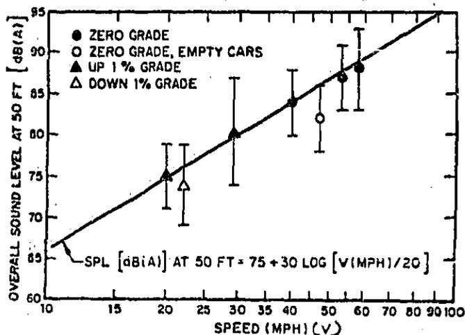
Figure 4-6. Wheel/Rail Noise Measured on Level Ground and on a 1% Grade
