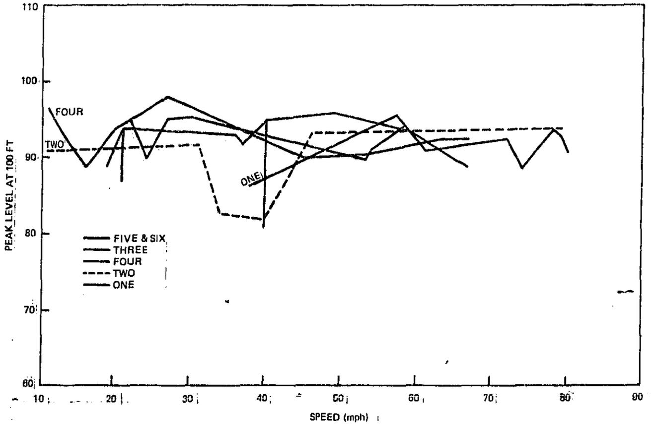
Figure 4-5. Relationship Between Maximum Noise Level and Number of Coupled Locomotives
