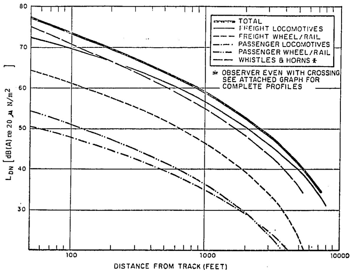
Figure 8-2. L<sub>DN</sub> vs Distance From Track for National Average Train Traffic
