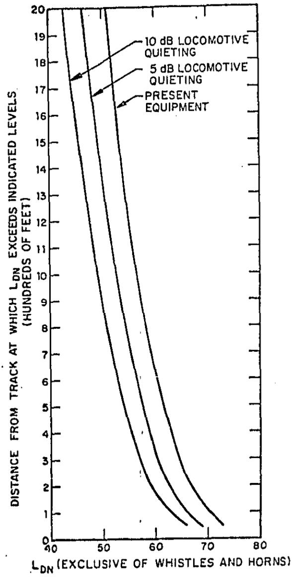
Figure 8-5. Distance From Track at Which Various L<sub>DN</sub> Occur Due to National Average Train Traffic
