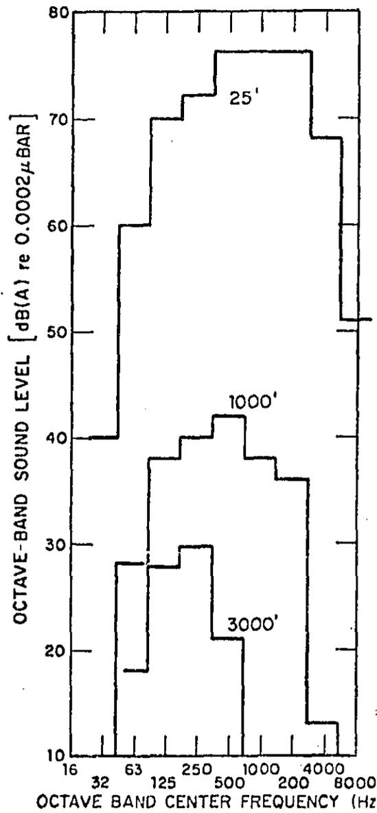
Figure 8-8. Influence of Frequency-Dependent Attenuations on Wheel/Rail Noise, Train No. 6, Region 2 (See Figure B.1.13 for Comparison)
