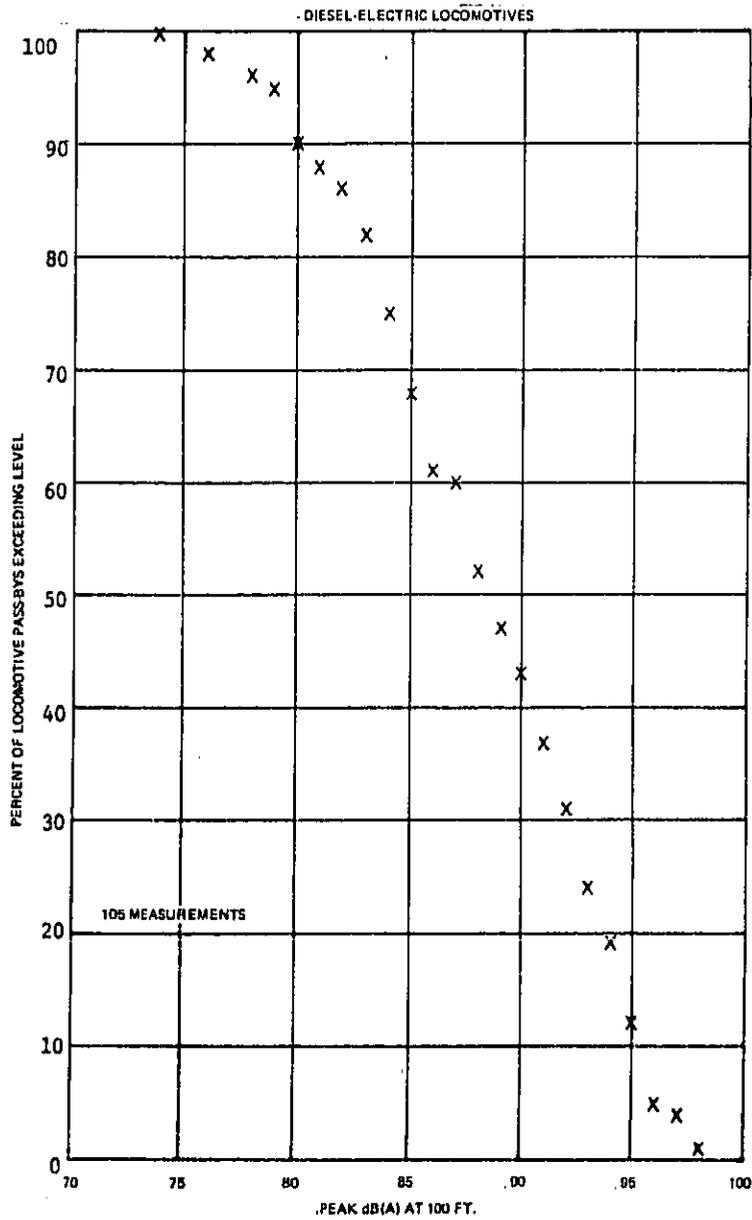
Figure 4-3. Diesel-Electric Locomotive Pass-Bys
