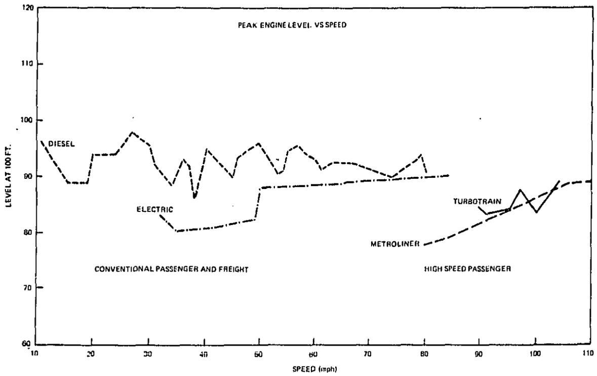
Figure 4-4. Peak Locomotive Noise Level vs. Speed
