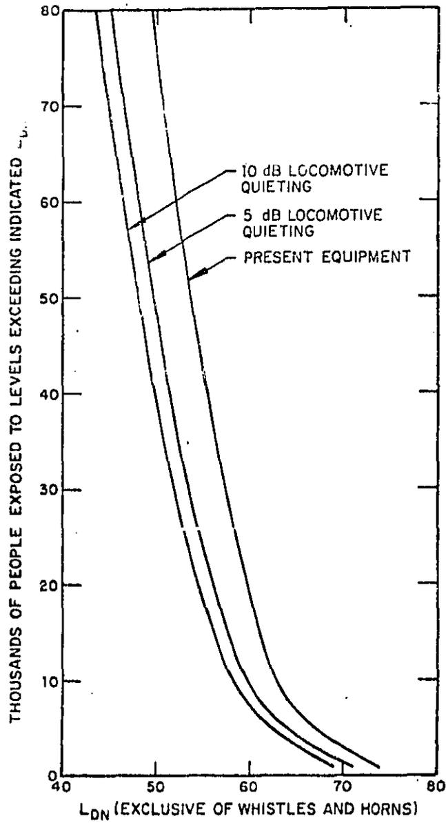
Figure 8-4. Thousands of People Exposed to Various L<sub>DN</sub> by 7.2 Miles of Track on the Dorchester Branch of the Penn Central
