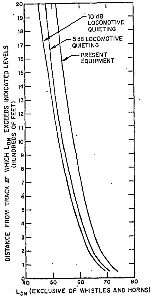
Figure 8-3. Distance From Track at Which Various L<sub>DN</sub> Occur Around the Dorchester Branch of the Penn Central
