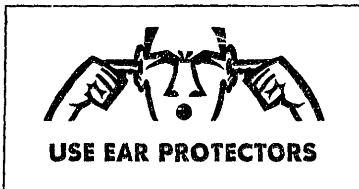
Figure V-1. Warning notice against hazardous noise. Color: black inscription on a yellow field. (Department of Employment, 1972)
