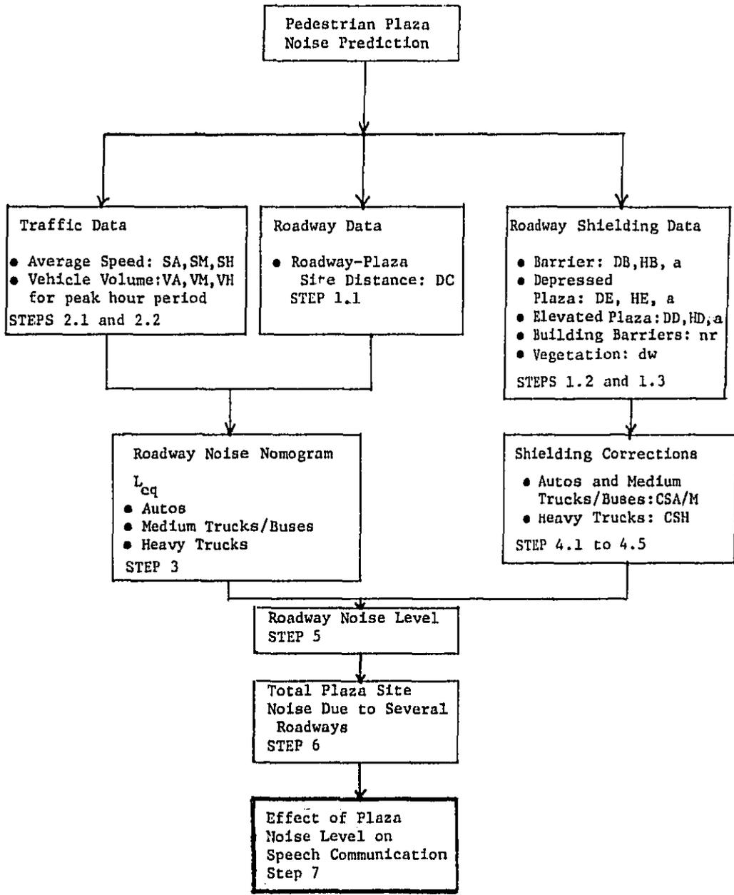
Figure 18. PLAZA NOISE PREDICTION FLOW DIAGRAM
