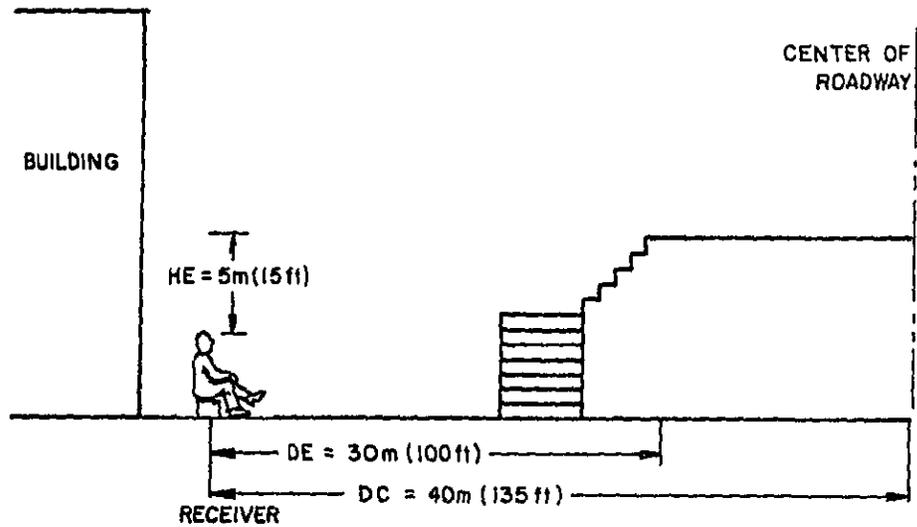
FIGURE 26 CROSS-SECTION OF PLAZA SHOWING ROADWAY #1
