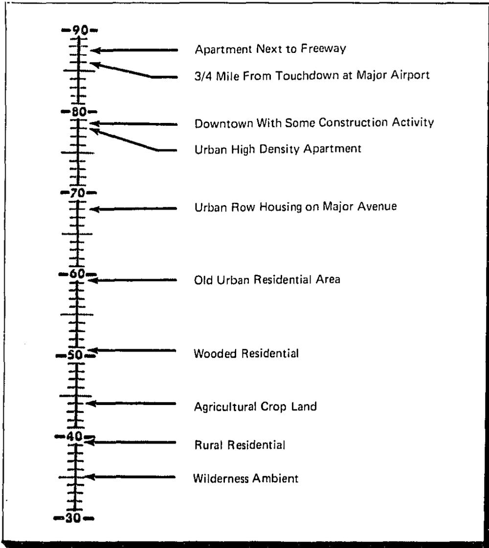
FIGURE 4. EXAMPLES OF OUTDOOR DAY-NIGHT AVERAGE SOUND LEVELS IN dB MEASURED AT VARIOUS LOCATIONS
