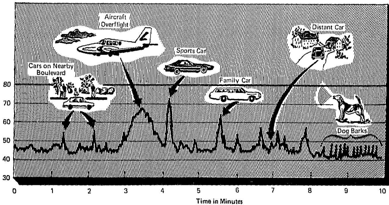
FIGURE 2. TYPICAL OUTDOOR SOUND MEASURED ON A QUIET SUBURBAN STREET
